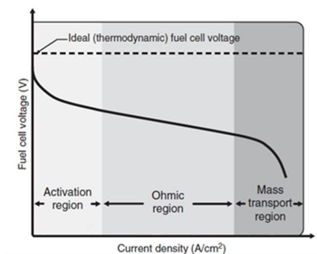
**Figure 2.4 : Typical I-V curve of a fuel cell [35].**
