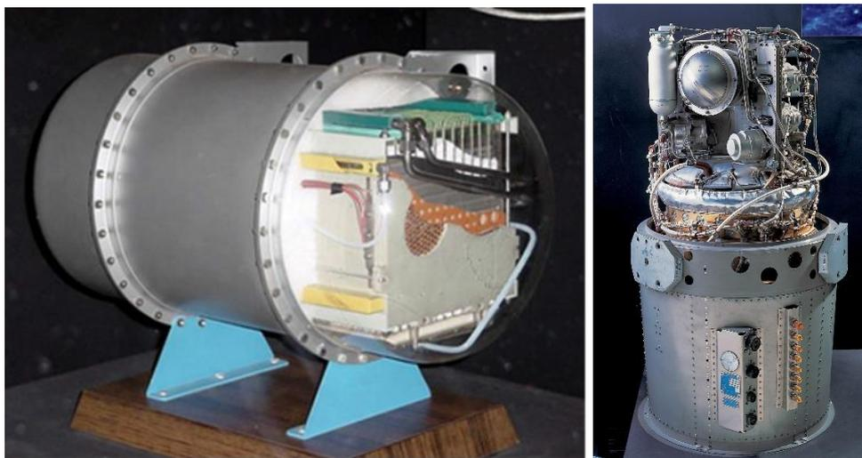
**Figure 2.2 :** Fuel cells used in Gemini (left) and Apollo space programs [29-30].
