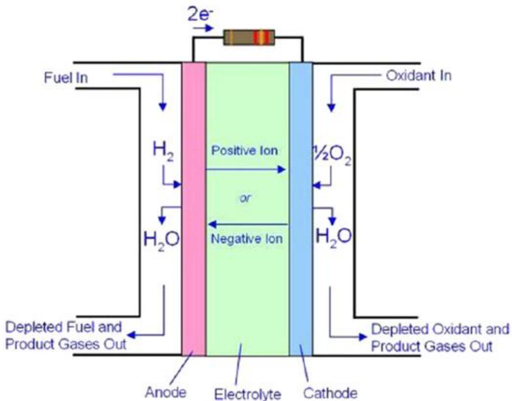
**Figure 2.3 :** Basic operation of fuel cells [33].
