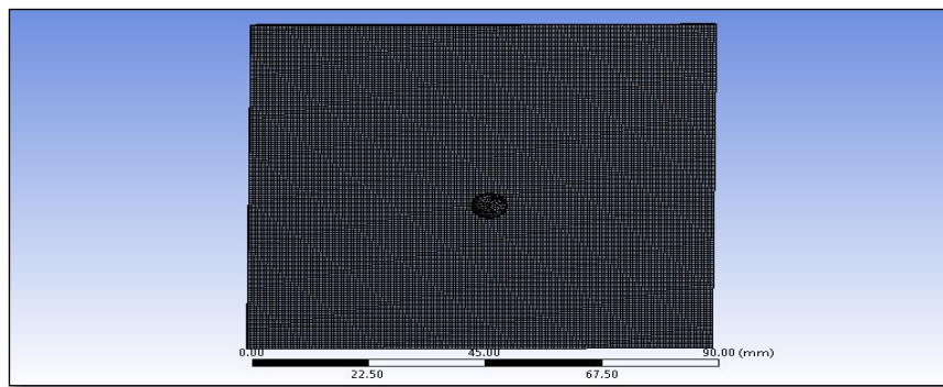
Figure 4.4: A portion of the target plate and rigid projectile mesh for finite-element simulation.
