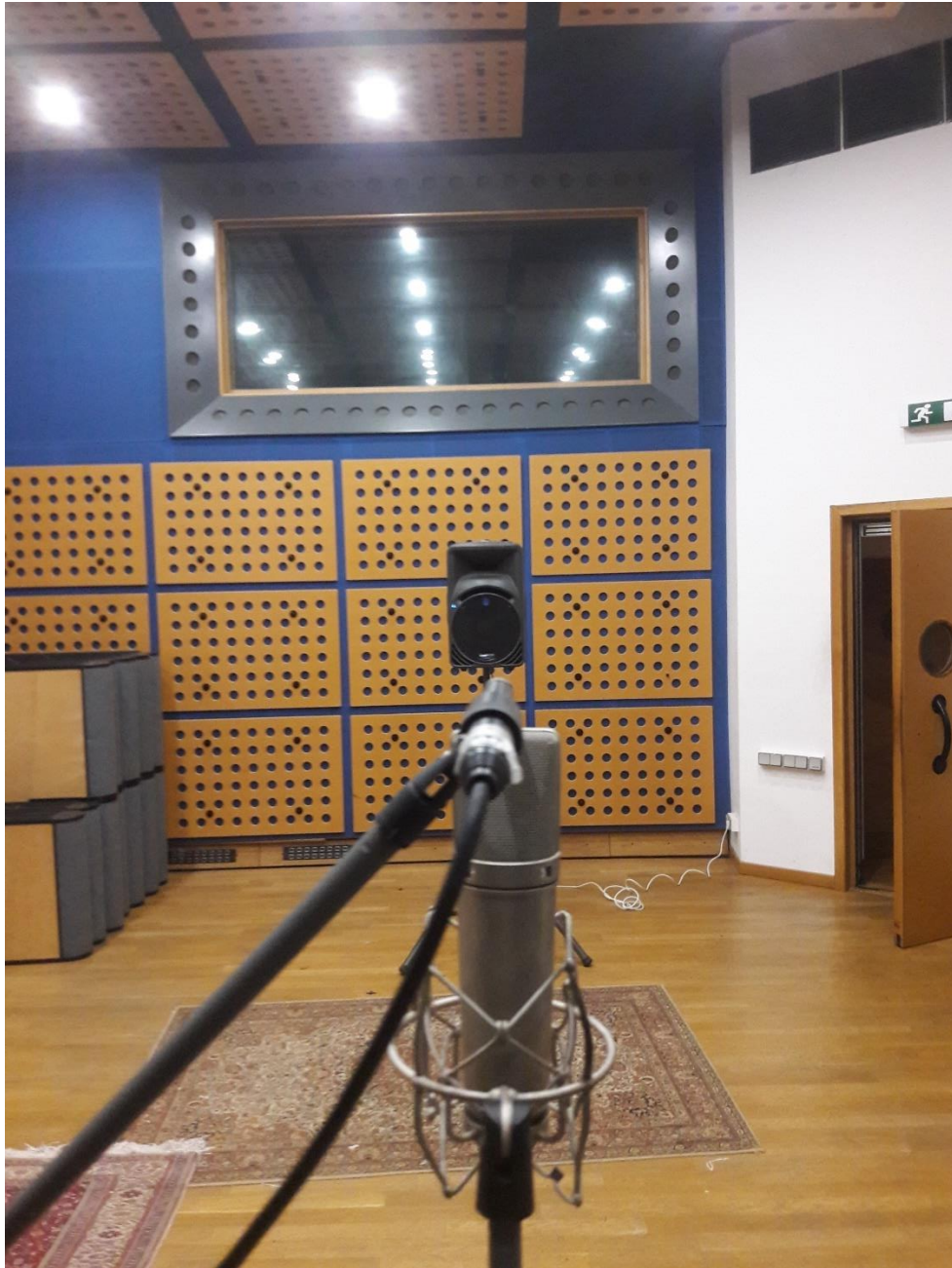
Figure D.1: Loudspeaker and microphone positions for DRR stimuli (# 2006) recording at 6 metres
