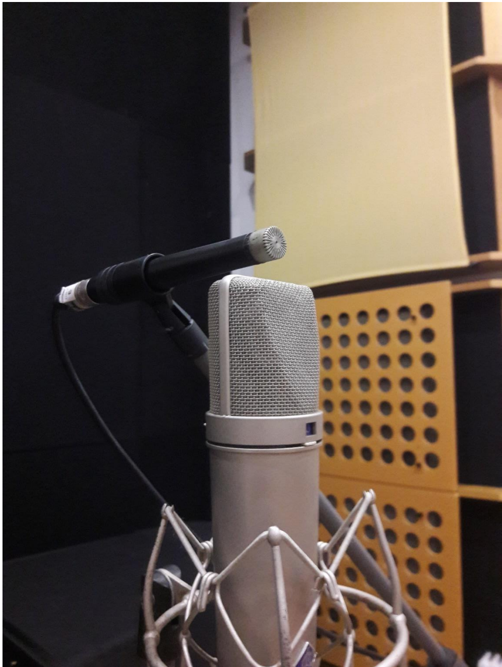
Figure D.3: Microphone setup (DPA was used for DRR and both cues stimuli recording, Neumann was used for intensity cue stimuli)
