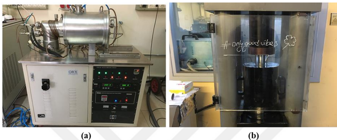
Figure 4.7 : Devices used for post-treatment: (a) Vacuum furnace, (b) CIP
