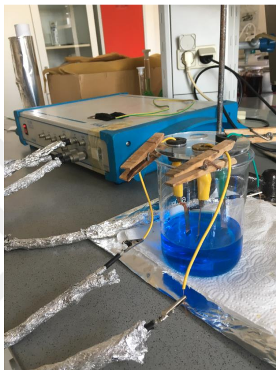
Figure 4.13 : Setup for plotting polarization curve in used electrolyte.
