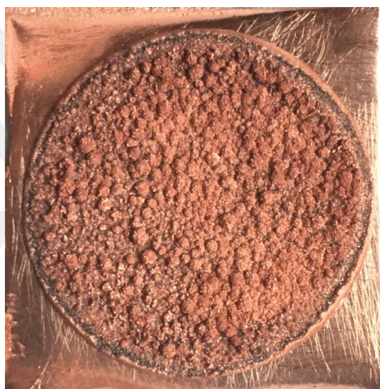
Figure 4.10 : Deposit fabricated by wetted SiC particles.
