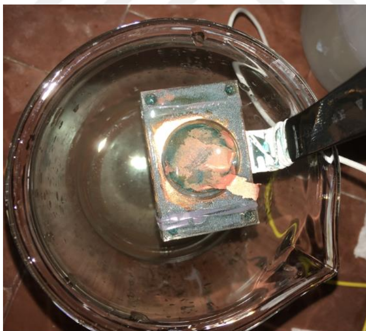
Figure 4.9 : Unsuccessful deposit fabricated by unwetted SiC particles.
