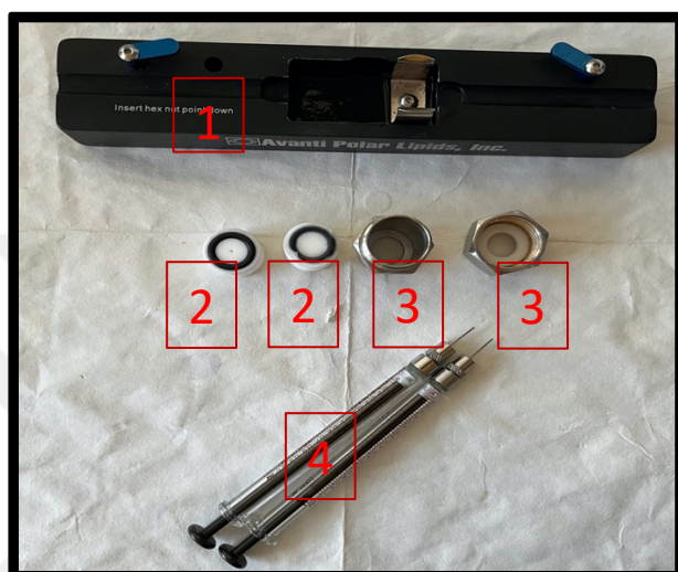
Figure 3.34 : The system for liposome and proteoliposome production. The number 1 is the mini extruder, number 2 is PTFE and number 3 is nut, number 4 is syringe respectively.
