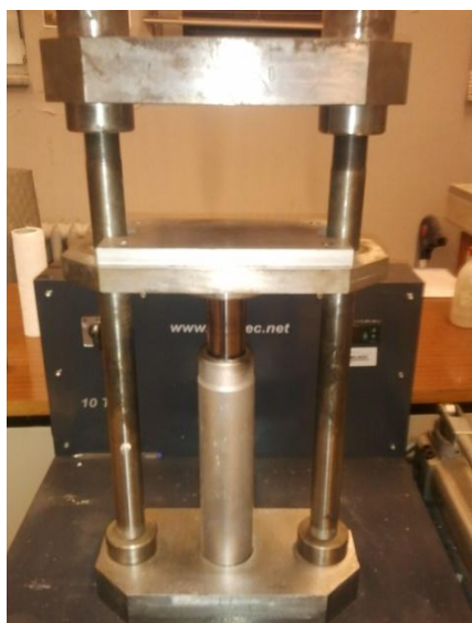
Figure 4.4: The Picture of MSE one-action hydraulic press.
