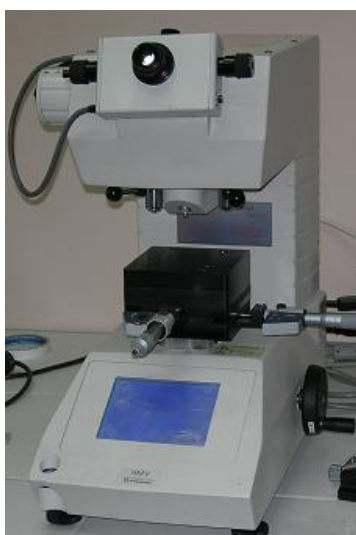
Figure 4.8: Shimadzu™ micro hardness tester.
