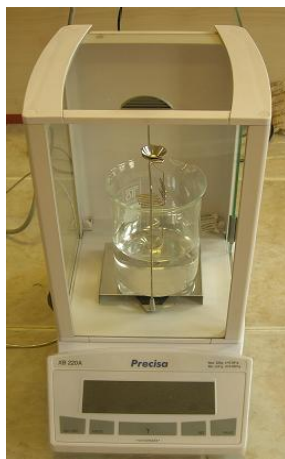
Figure 4.7: Precisa™ XB220A sensitive balance with the Archimedes kit.
