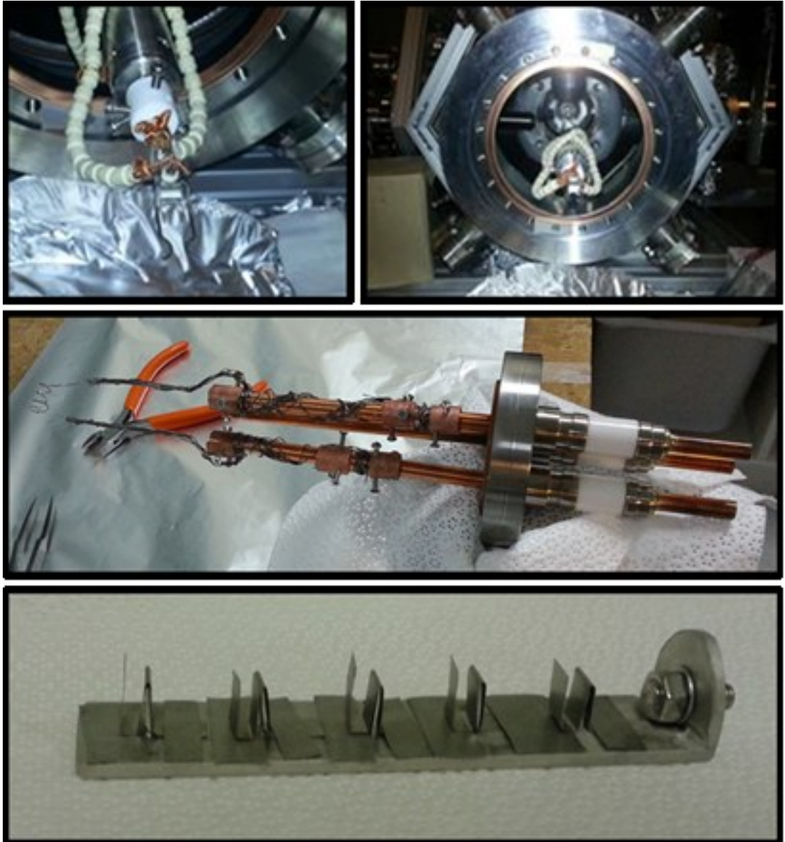
Figure 2.7 : Additional homemade parts of UHV system. Sample fork (upper images), Pt evaporator (middle) and sample carrier (bottom).
