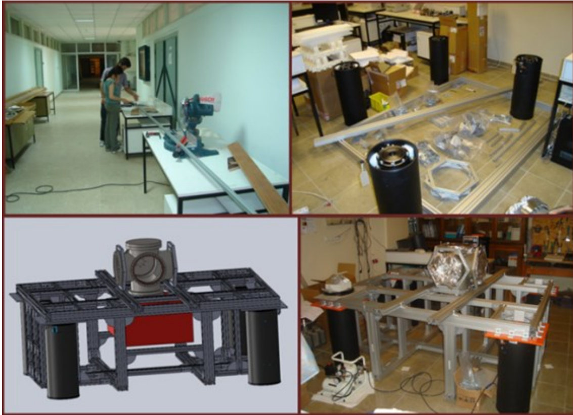
Figure 2.8 : Making the vibration isolation table. Preparation of the isolation system (upper images), drawing of the table (bottom-left) and the table itself (bottom-right)
