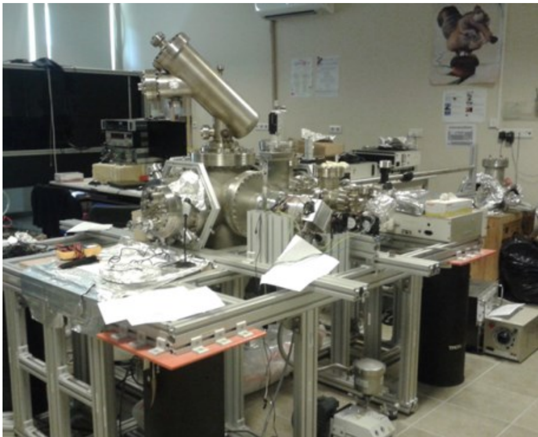
Figure 2.4 : Photo of UHV system on its frame in our laboratory which was constructed during this study.
