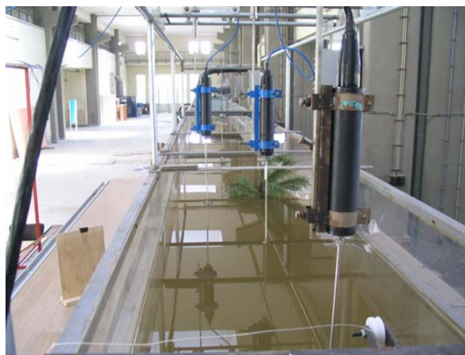
Figure 4.3: The centerline view of the flume and the Acoustic Doppler Velocimeters
