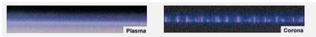
Figure 1.20 : Visual difference between plasma and corona ( www.enerconind.com )
