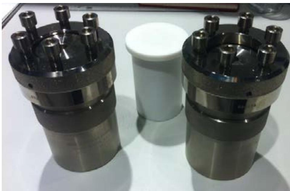
**Figure 2.3 :** Static autoclave systems.
