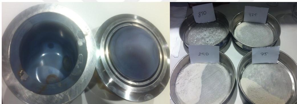
**Figure 2.1 :** a) ball mill mortar used to grind recycling glass, b) various sieves and sieved recycling glasses.
