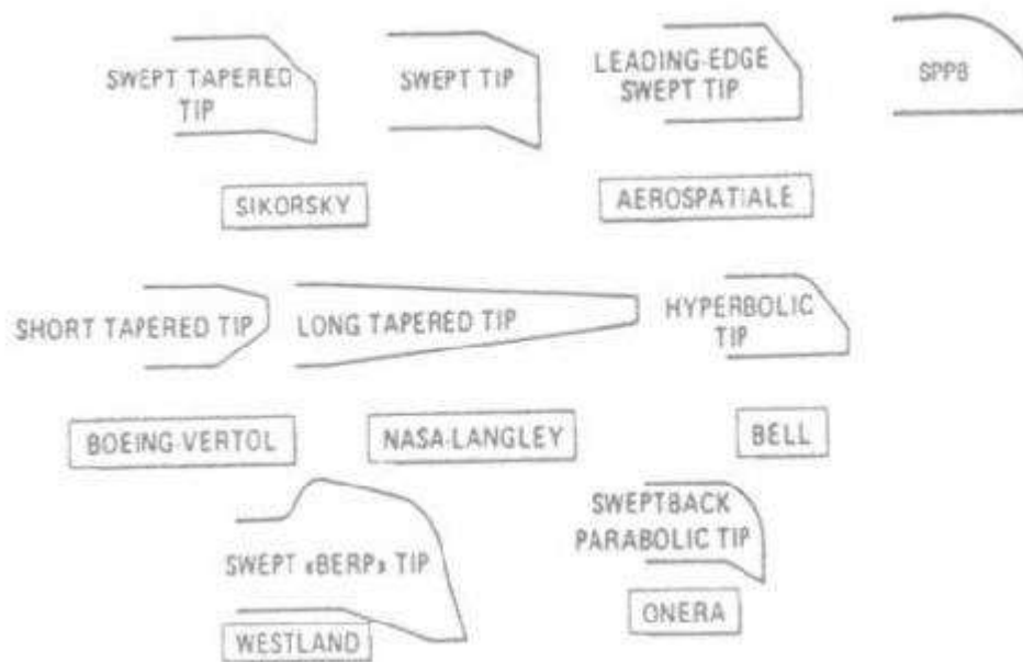
Figure 3.1 Examples of Blade Tips Either Already Produced or Under Development [18]
