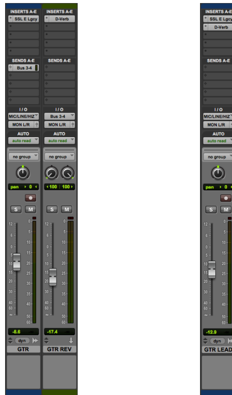
Figure 3.1: Send and return model (on the left) vs. Insert (on the right)
