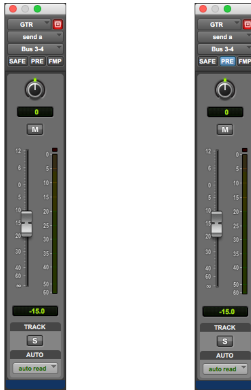
Figure 3.3: Post-fader (on the left) vs. Pre-fader (on the right)
