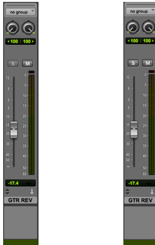
Figure 3.2: Solo isolate (on the left) vs. normal aux usage (on the right)
