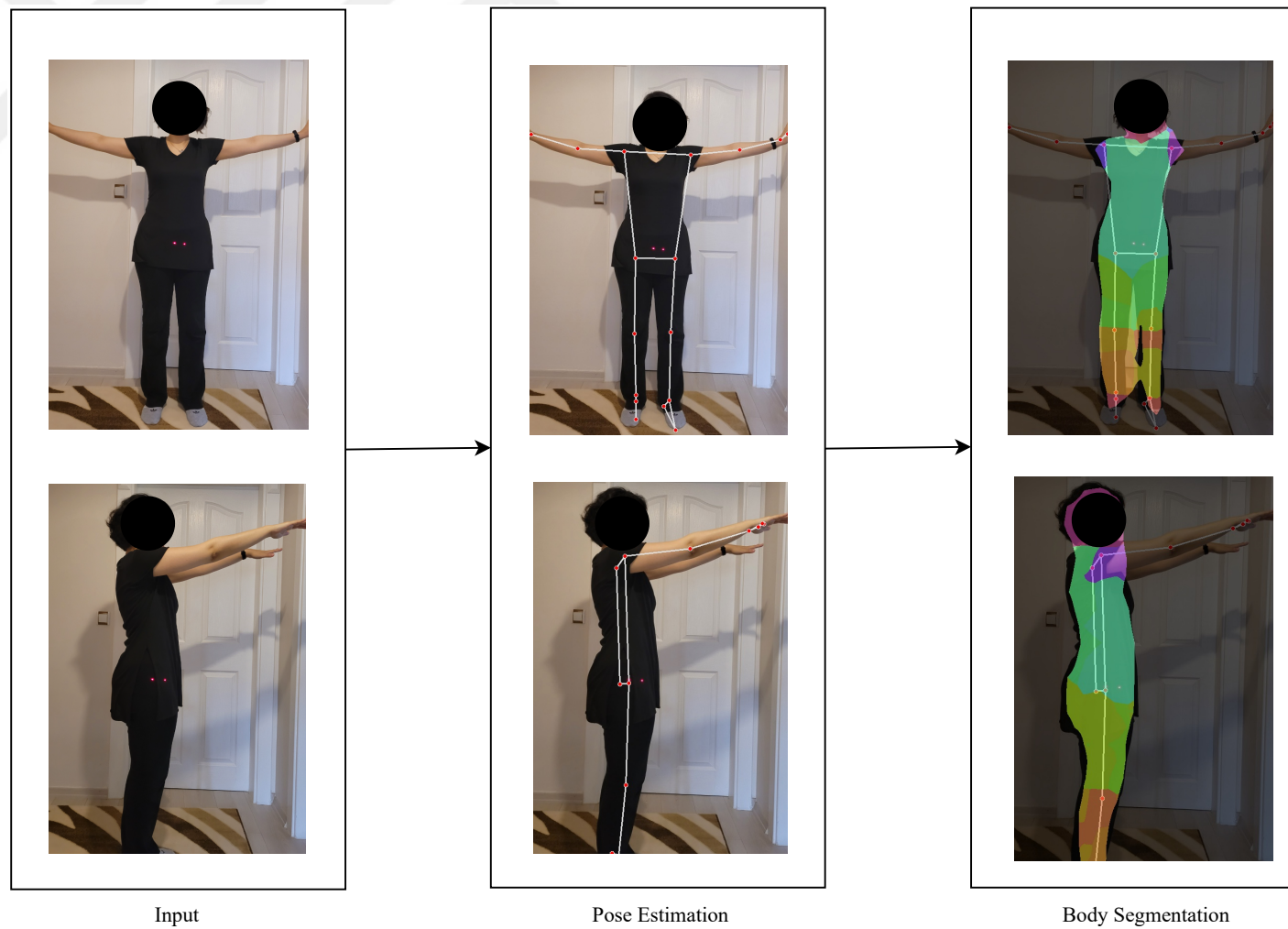
Figure 3.4 : Sample input images and the masks created by the pose estimation and the body segmentation models.
