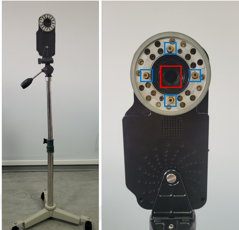
Figure 3.2 : Camera Version 2. On the left, the whole system, including the tripod. On the right the camera and laser setup. Blue squares show the laser points, the red square shows the location of the camera.
