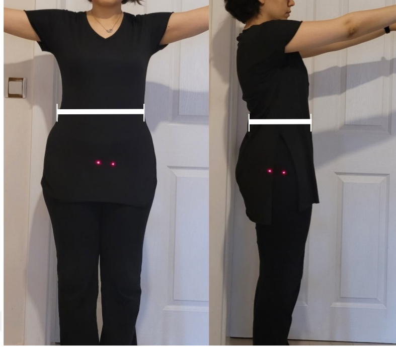
Figure 3.7 : Major (on the left) and minor (on the right) axes of the assumed ellipse on the human subject.
