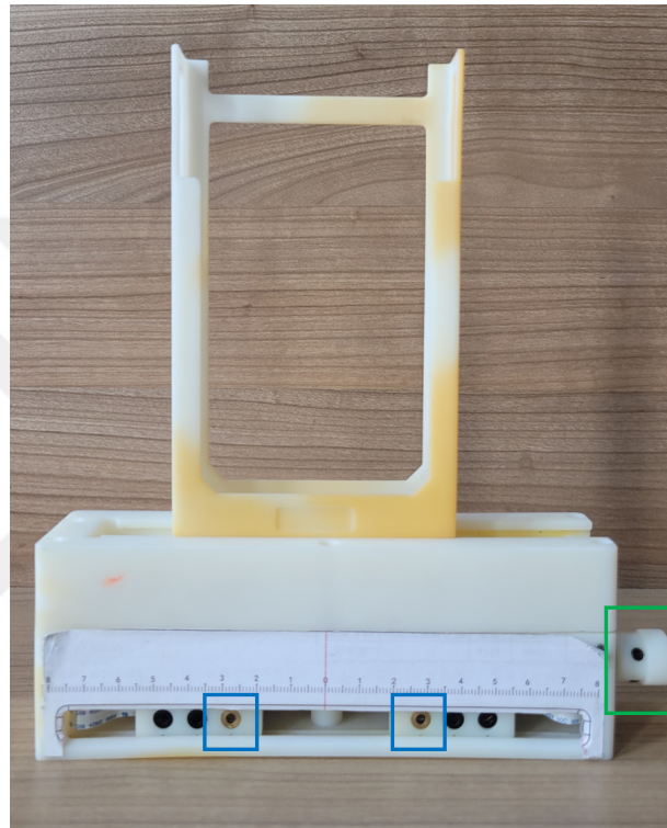
Figure 3.1 : Camera Version 1. Blue squares indicate the locations of laser points, green rectangle shows the adjusting wheel.
