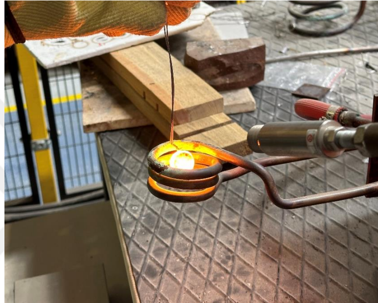
Figure 4.1 : General view of induction heating.
