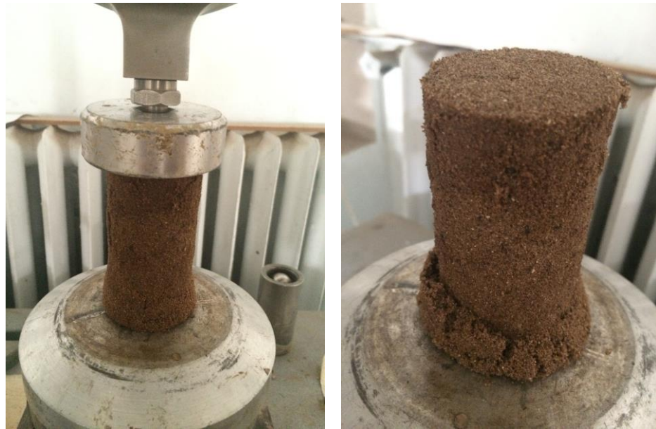
Figure 5.12: Unconfined axial test 7 th Day reinforced sand with 3% of P.B
