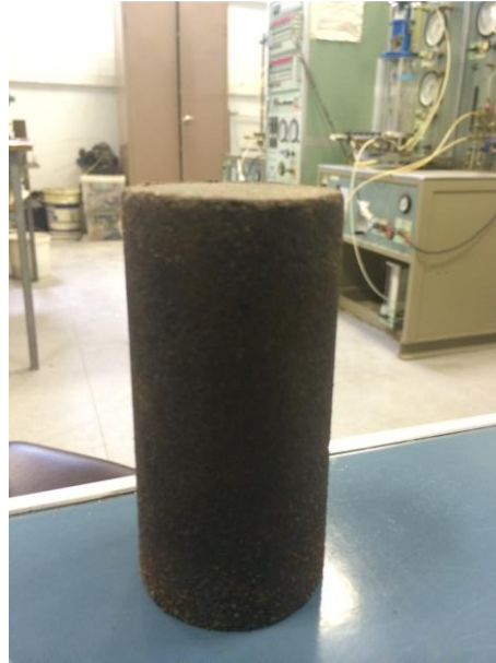
Figure 5.5: Dynamic triaxial test 1 st day reinforced sand with 10% of P.B
