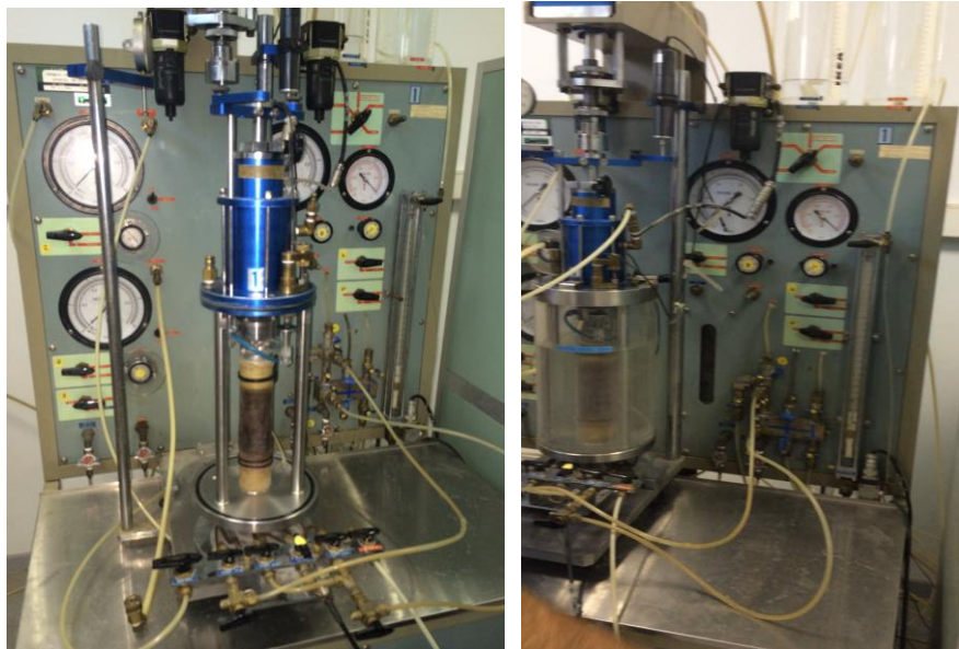
Figure 5.4: Digital system of the triaxial apparatus
