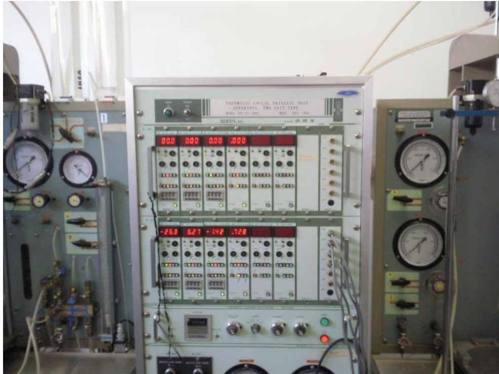
Figure 5.4: Digital system of the triaxial apparatus
