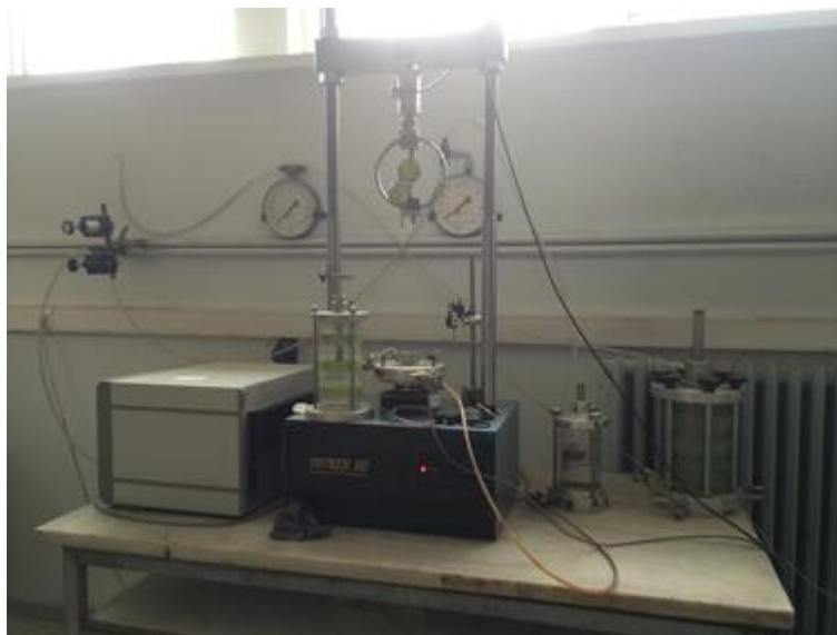
Figure 5.14: Triaxial Test Apparatus in ITU Soil Dynamics Laboratory
