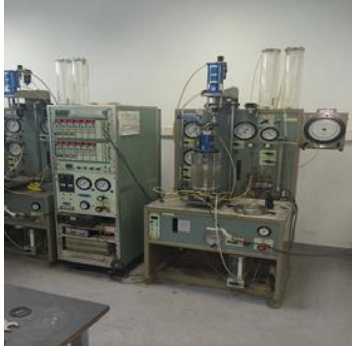
Figure 5.2: Dynamic triaxial Test Apparatus in ITU Soil Dynamics Laboratory
