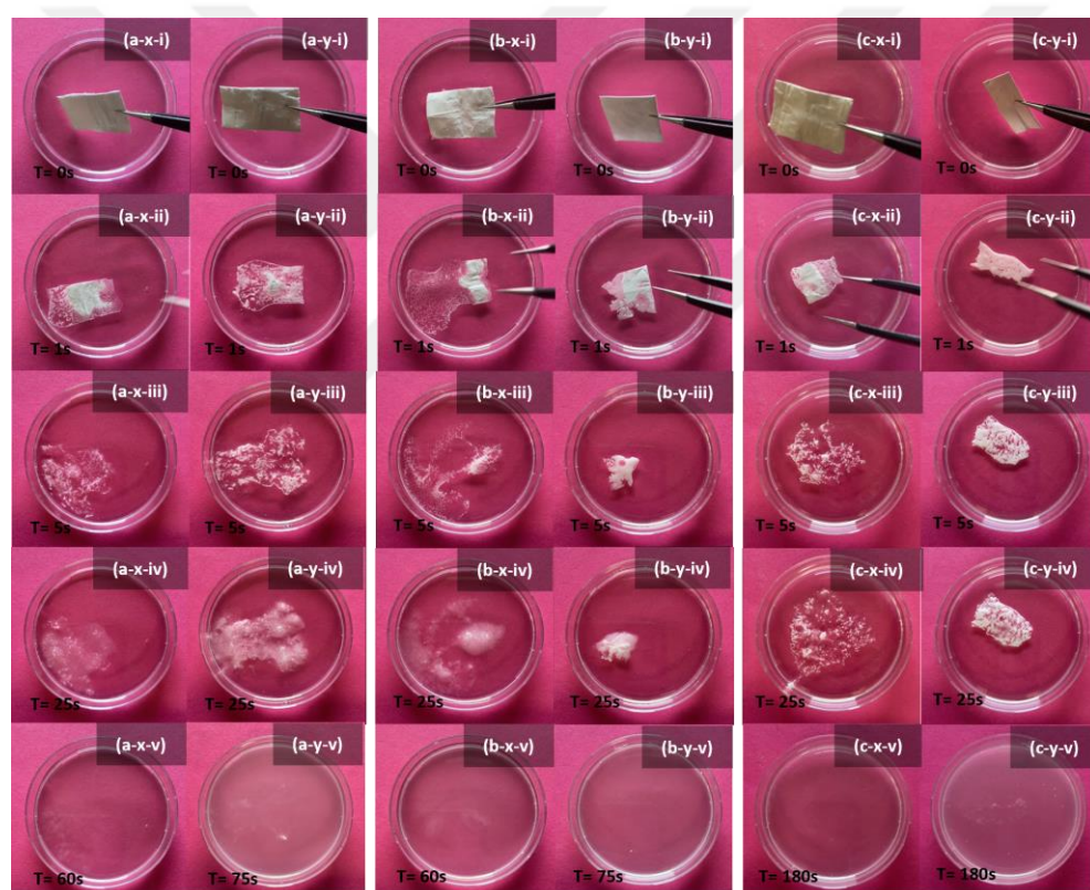
Figure 4.14: The progressive dissolution behavior of electrospun mats comprising of (a) Pul/E2/HP- \beta -CD IC, (b) Pul/E2/HP- \gamma -CD IC, (c) Pul/E2 at different drug:CD (x) 0.5:1 and (y) 1:1 stoichiometries in simulated saliva over time.
