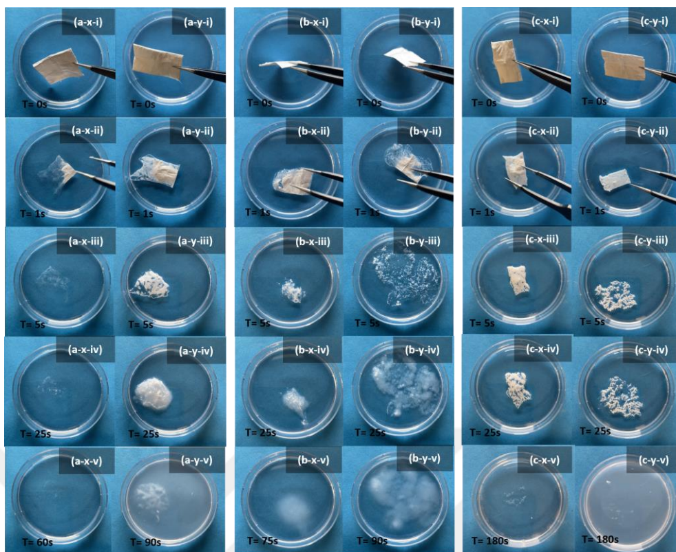
Figure 4.22: The progressive dissolution behavior of electrospun mats comprising of (a) Pul/E3/HP-β-CD IC, (b) Pul/E3/HP-γ-CD IC, (c) Pul/E3 at different drug:CD (x) 0.5:1 and (y) 1:1 stoichiometries in simulated saliva over time.
