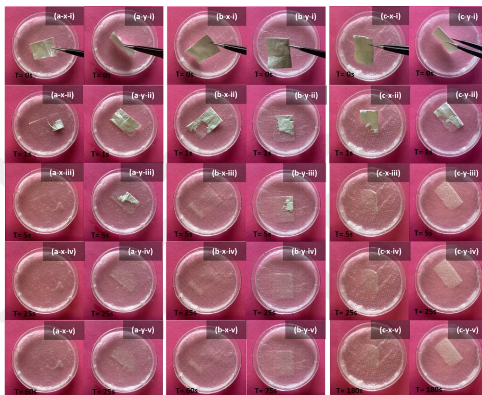
Figure 4.15: The progressive dissolution behavior of electrospun mats on tissues wetted with simulated saliva. (a) Pul/E2/HP- \beta -CD IC, (b) Pul/E2/HP- \gamma -CD IC, (c) Pul/E2 at different drug: CD (x) 0.5:1 and (y) 1:1 stoichiometries in simulated saliva over time.
