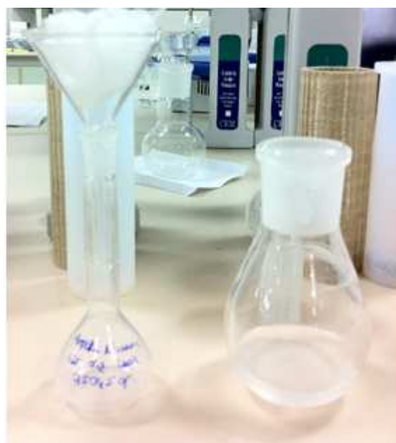
Figure 3.5 : Glass wool filtration.
