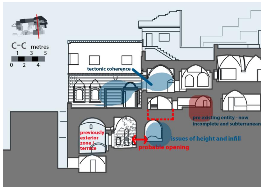
Figure 3.8 : Schematical mapping of the sectional characteristics of Block-I in the north-south direction.
