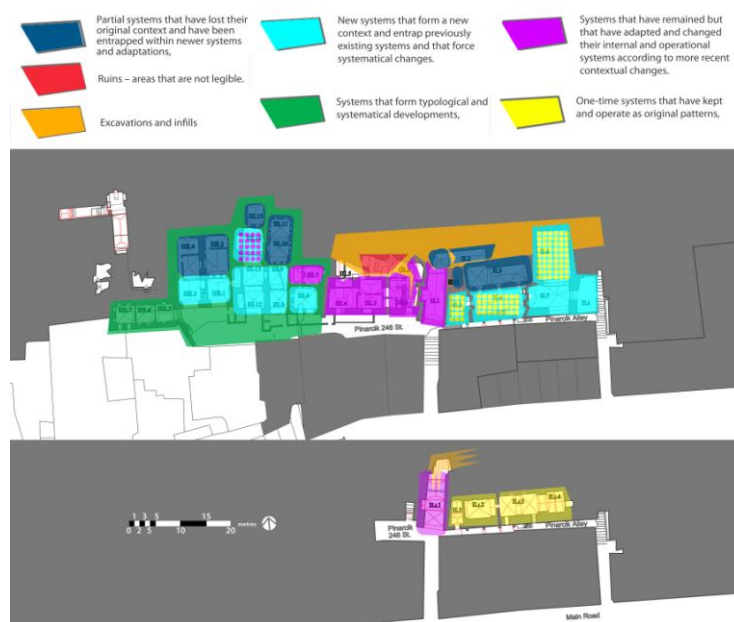
Figure 3.1 : Mapping of the characteristics of the upper layer.
