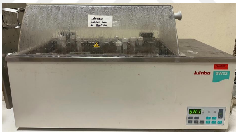
Figure 3.3 : Shaking water bath instrument used for physical adsorption.
