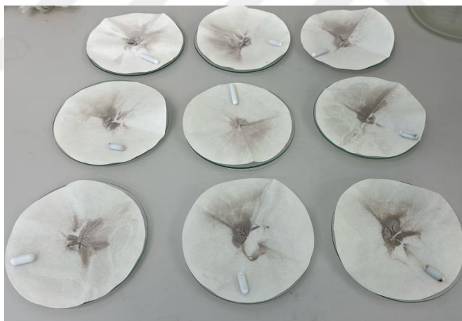
Figure 3.5 : Immobilized enzyme that has been filtered following immobilization via physical adsorption.
