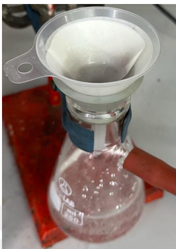
Figure 3.4 : Apparatus used for filtration.
