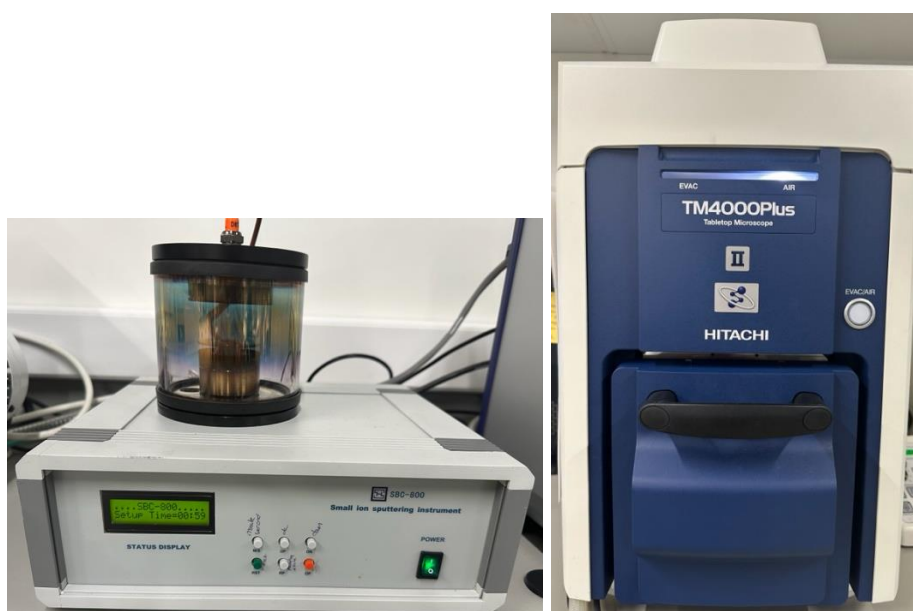
Figure 3.9 : SEM and its coater instrument used for characterization.
