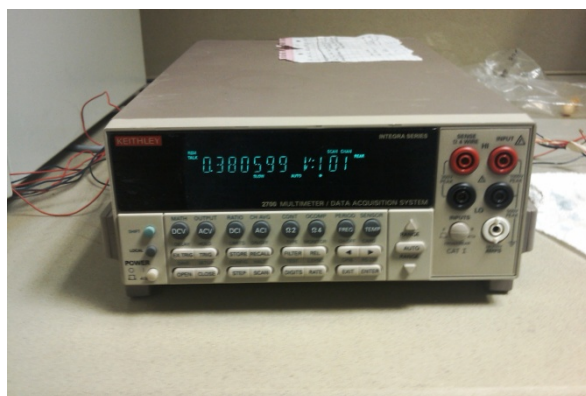
Figure 3.2: Multimeter with a data acquisition system (Keithly 2700, Cleveland, OH, USA).
