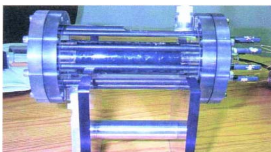
Figure 2.4: Single Chamber MFC reactor
