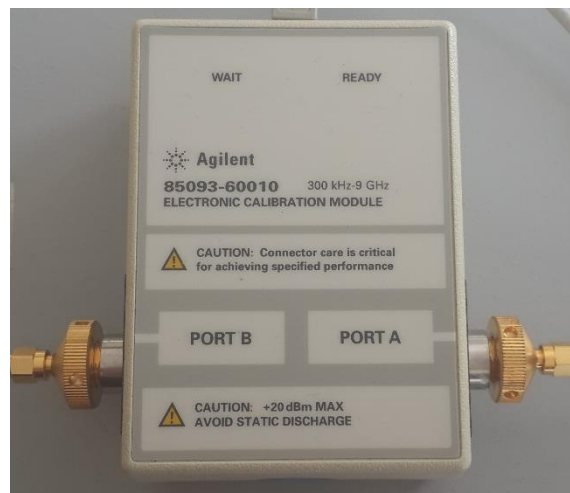
Figure 5.4 : Electronic calibration module Agilent/HP 85093C, utilized for calibrating vector network analyzer.
