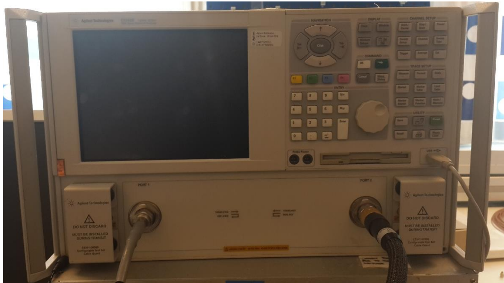
Figure 5.1 : The network vector analyzer Agilent E8362 B, used to perform measurements.
