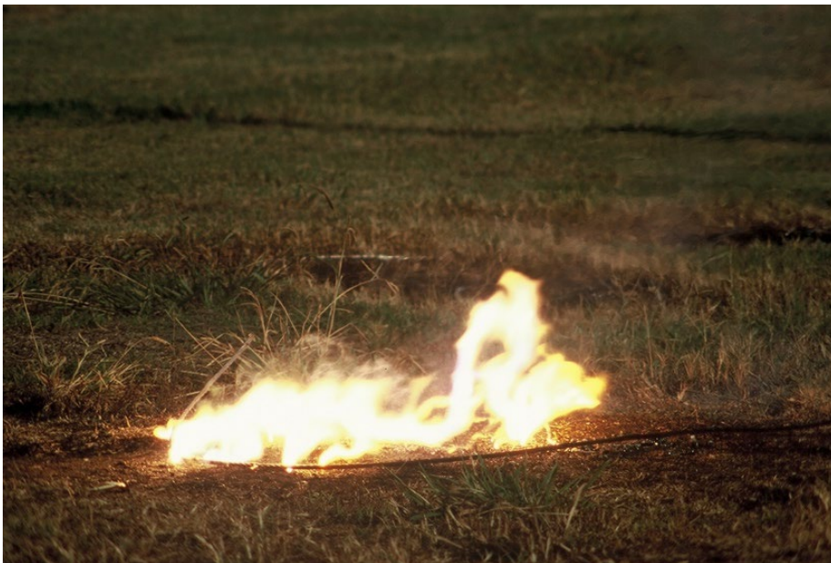
Figure 2.2 : Energized downed conductor implemented by Texas A&M University [17]
