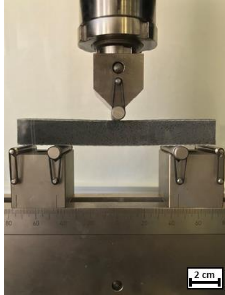
Figure 2.3 : Three-point bending test specimens of foam-filled I-beam composites.
