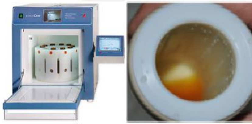
Figure 4.5 : Microwave digestion instrument (Milestone, Model Ethos One) and digestion vessels after digestion.
