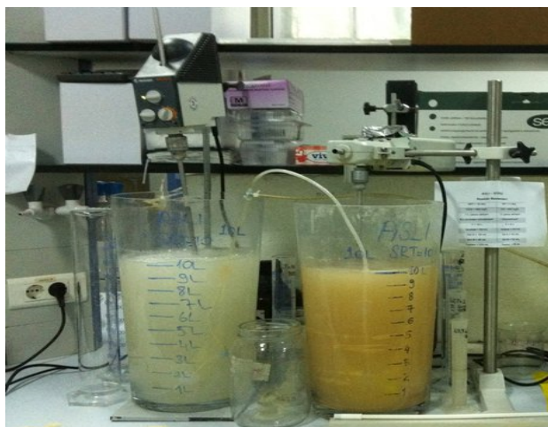
Figure 3.1 : Picture of the SBRs, both control (right) and antibiotic (left).
