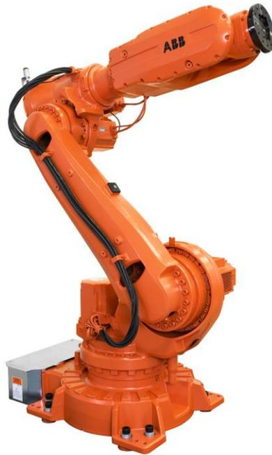
**Figure 6.1 :** ABB IRB 6620 (Floor mounted) [35].
