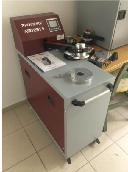
Figure 4.20: Air permeability test device.
