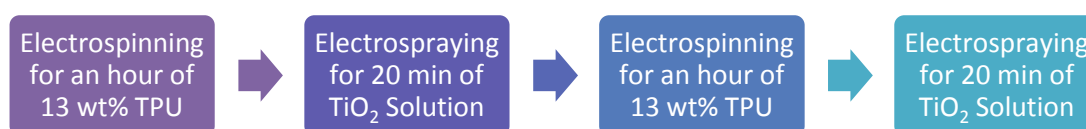
Figure 4.12: Schematic of fabrication of sandwich structure.
