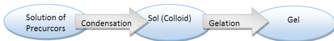
Figure 4.13: Sol-Gel preparation process.
