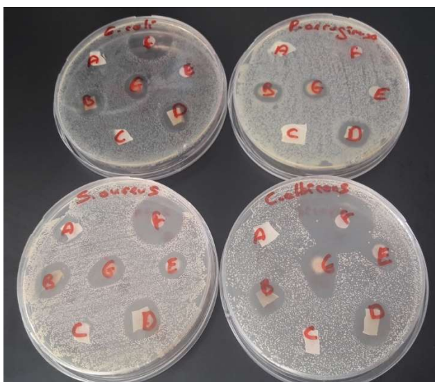
Figure 4.66 : Observed inhibition zones of A: PAN nanofiber, B: PAN/Ag nanofiber (prepared from 20 wt % \text{AgNO}_3 ), C: P (AN-co-IA) nanofiber, D: P (AN-co-IA)/Ag nanofiber (prepared from 20 wt % \text{AgNO}_3 ), E: PAN powder, F: P (AN-co-IA) powder and G: \text{AgNO}_3 powder against four different microbial culture in plates.
