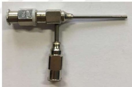
Figure 3.4 : The coaxial needle (Raméhart Custom Needle, 100-10-COAXIAL-2016).
