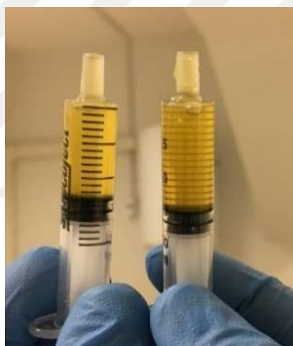
Figure 4.50 : PAN/Ag polymer solutions prepared from 10 wt % \text{AgNO}_3 (left) and 20 wt % \text{AgNO}_3 (right) after stirring of 10 days.
