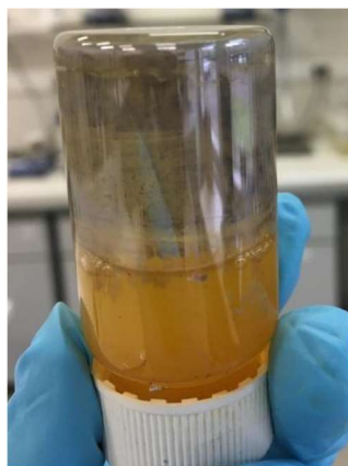
Figure 3.9 : Image of silver-mirror reaction of Ag-PDMPy.
