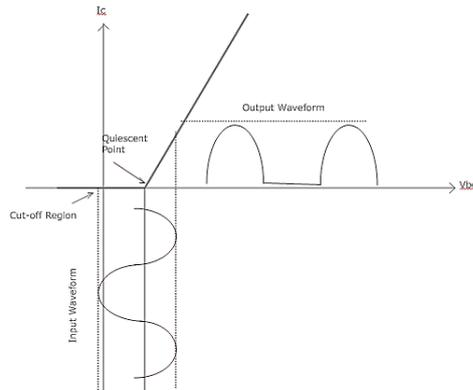
**Figure 2.39 :** The Class B power amplifier input and output signals.
