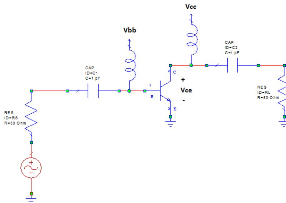
**Figure 2.46 :** A generic power amplifier circuit.
