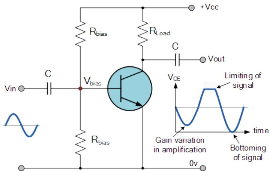
**Figure 2.15 :** Amplifier circuit distortion [Url-6].
