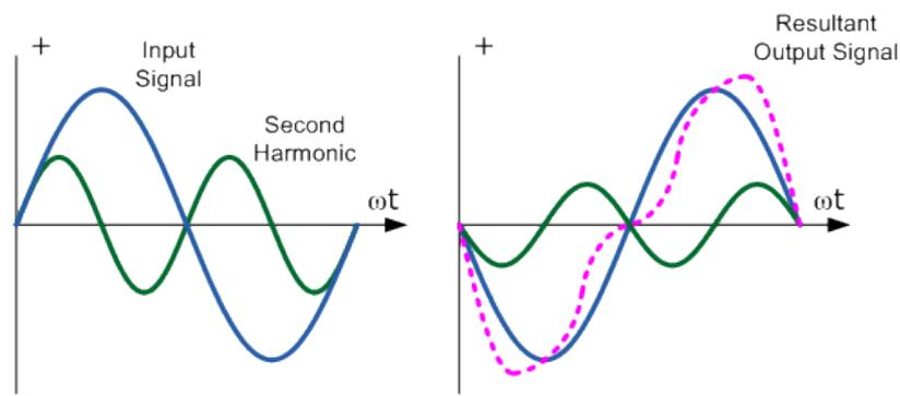
**Figure 2.17 :** Frequency distortion due to harmonics [Url-6].
