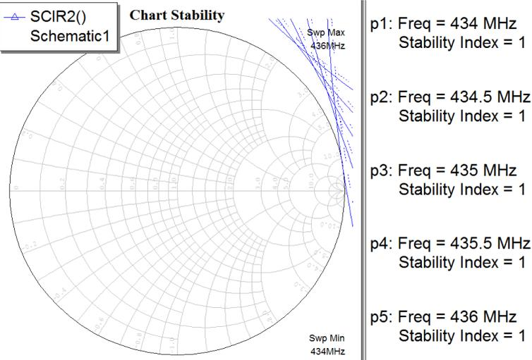
Figure 2.12 : The output stability circles.
