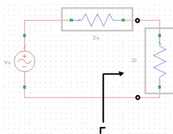
**Figure 2.28** : Simple circuit configuration showing measurement location of reflection coefficient.
