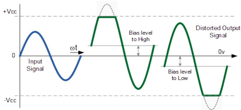
**Figure 2.16 :** Amplitude distortion due to incorrect biasing [Url-6].
