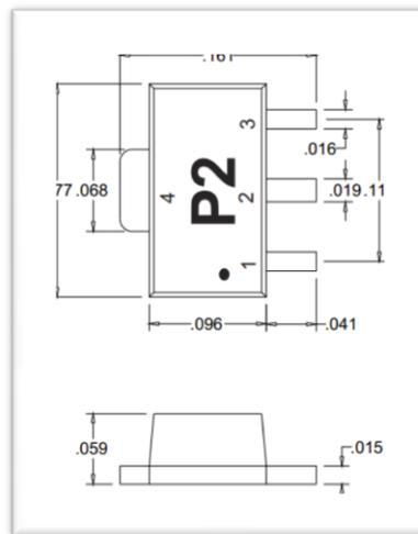
**Figure A.1 : Transistor dimensions in inch.**
