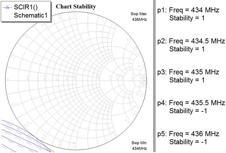
Figure 2.11 : The input stability circles.
