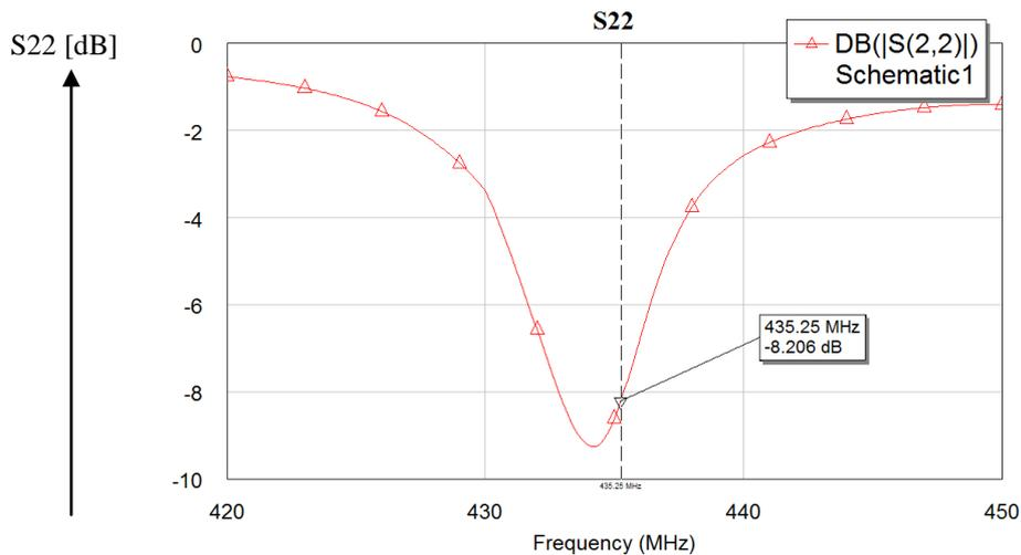
**Figure 2.25 :** The power amplifier's  $S_{22}$  graph.
