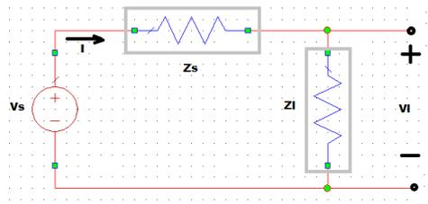
**Figure 2.51 :** The source and load impedance.
