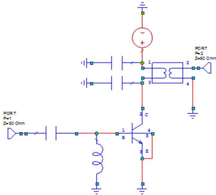
**Figure 2.43 :** The Class C power amplifier schematic.
