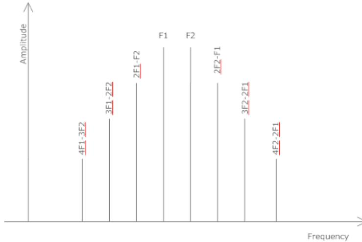
**Figure 2.20** : Two tone intermodulation products.
