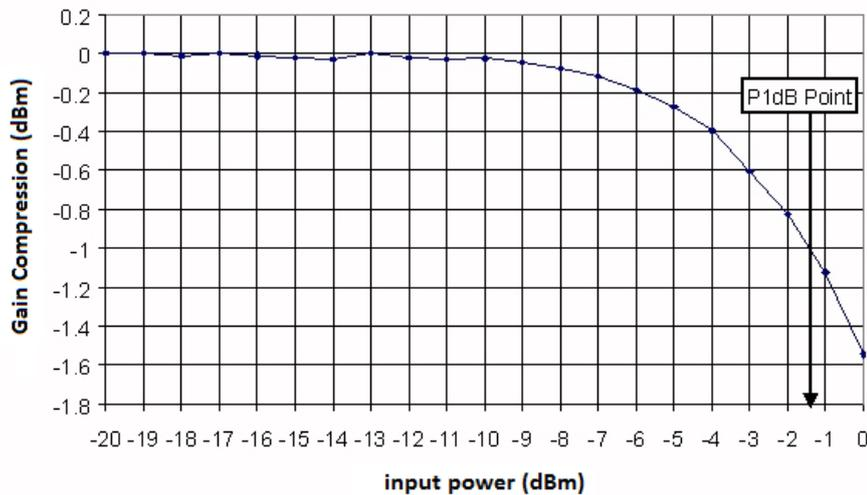
**Figure 2.6** : Alternative technique for 1 dB compression point [Url-14].
