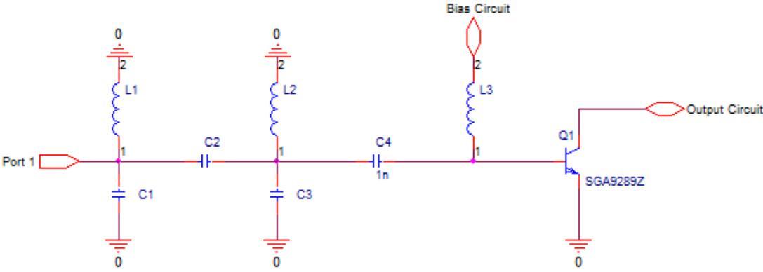
**Figure 2.54 :** The input matching circuit.
