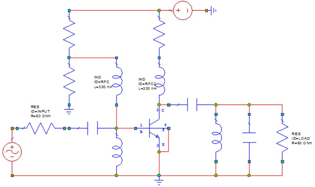
**Figure 2.35 :** The basic schematic version of Class A.
