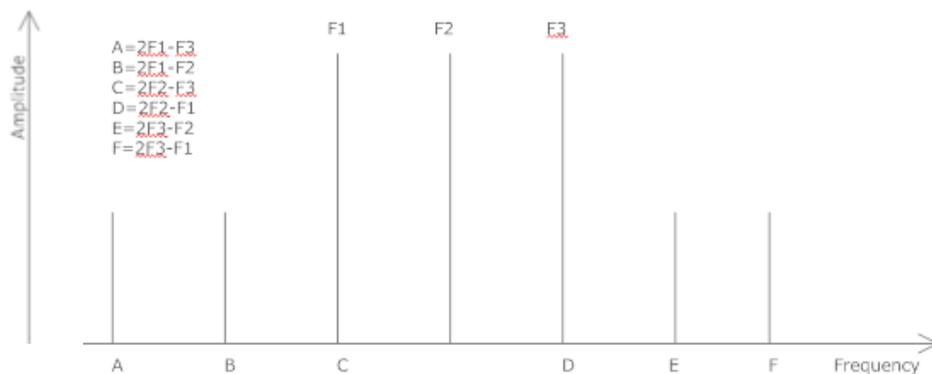
**Figure 2.19** : Three tone intermodulation products.
