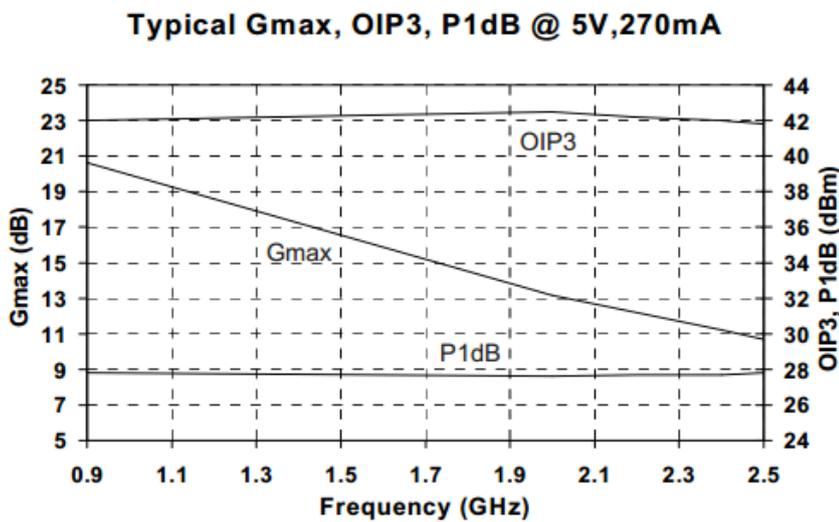
**Figure 3.3 :** The gain, P1dB and OIP3 graph (SGA9289Z Medium Power Discrete SiGe Transistor Datasheet, 2006).
