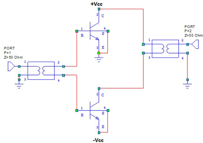
**Figure 2.38 :** The Class B push-pull power amplifier.
