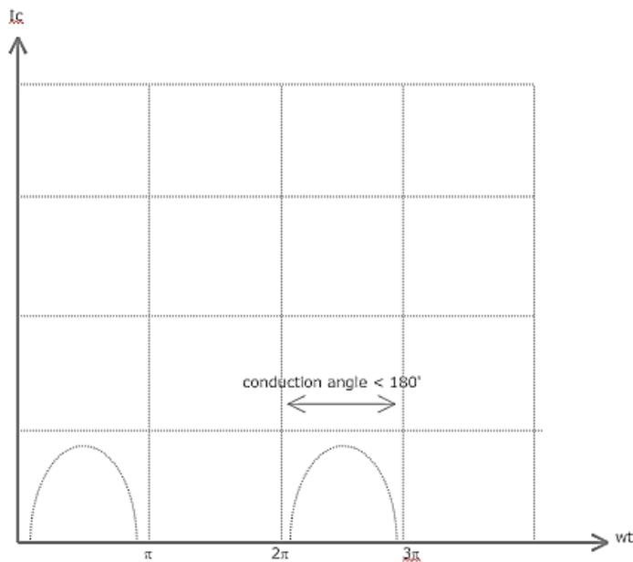
**Figure 2.44 :** The Class C power amplifier conduction angle.
