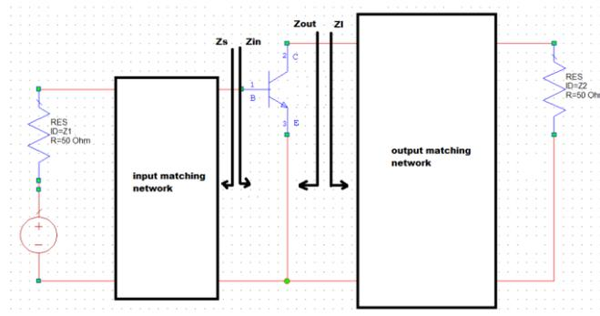
**Figure 2.52 :** An amplifier schematic showing  $Z_{in}$ ,  $Z_{out}$ ,  $Z_L$  and  $Z_S$ .
