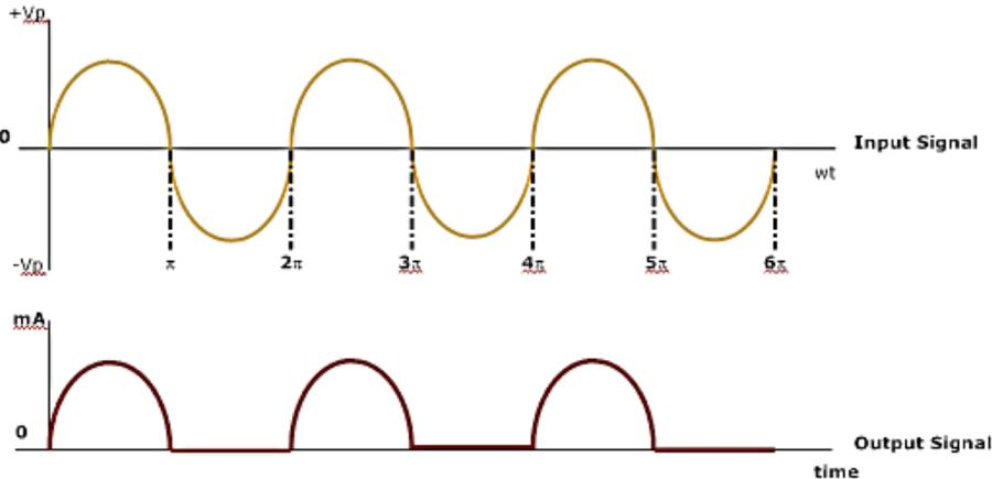
**Figure 2.37 :** The conduction angle for Class B power amplifier.
