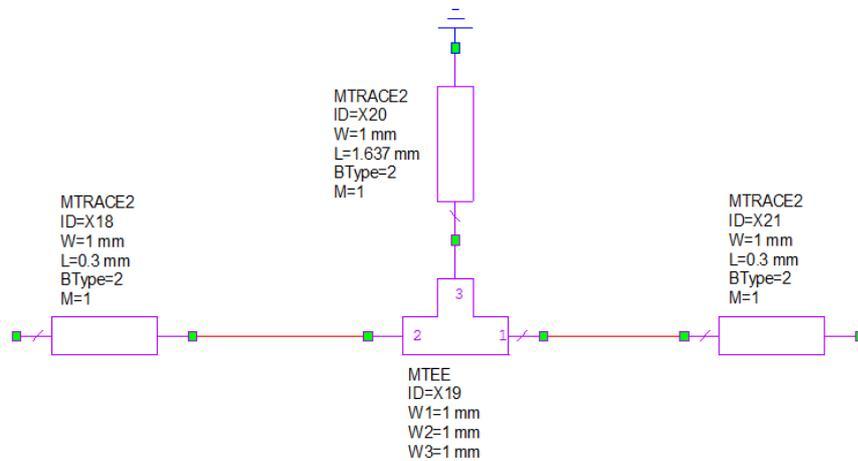
**Figure 3.1 :** The transmission lines.
