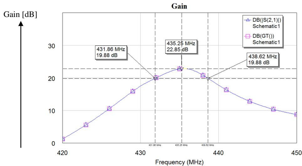
**Figure 2.23** : Gain with  $G_T$  and  $S_{21}$ .
