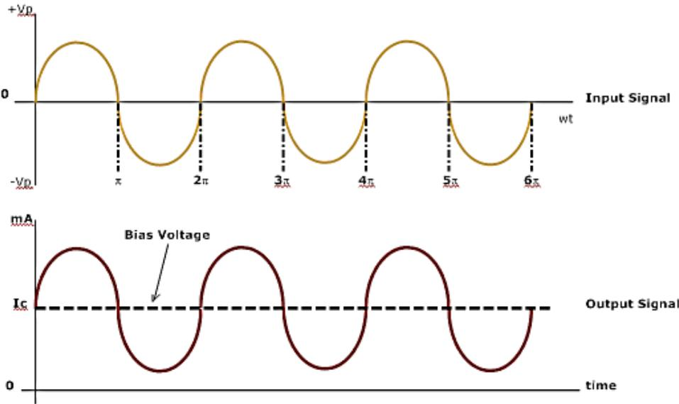
**Figure 2.34 :** Class A input and output wave form.
