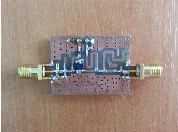
**Figure 3.11 : PCB with Components.**
