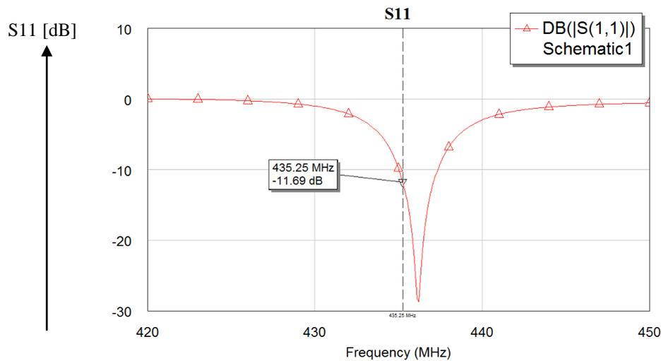
**Figure 2.24 :** The power amplifier's  $S_{11}$  graph.
