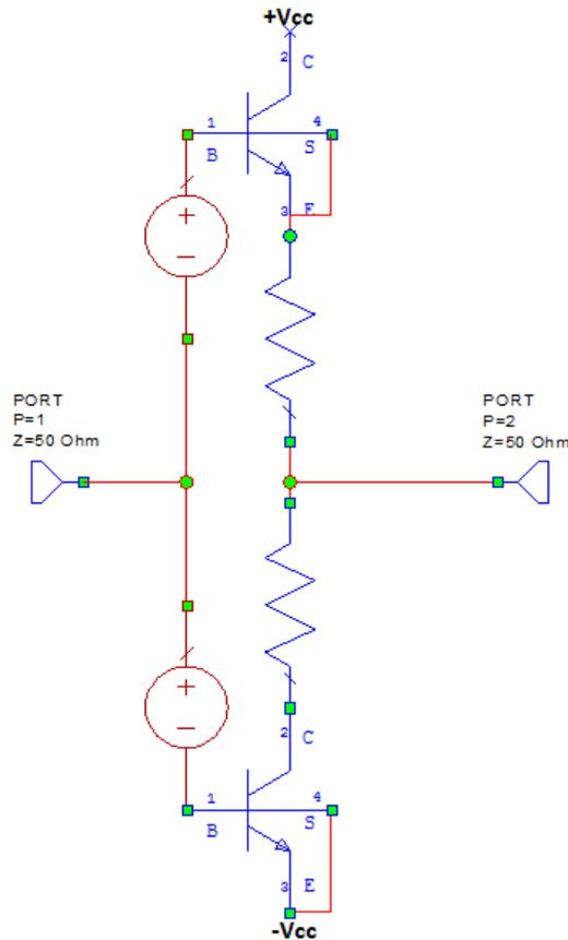
Figure 2.42 : The Class AB schematic.
