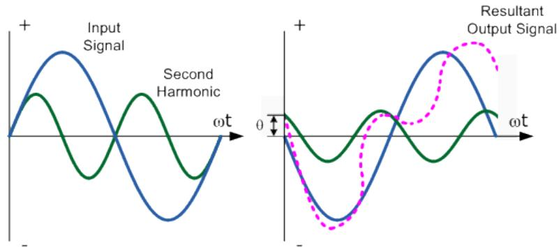
**Figure 2.18 :** Phase distortion due to delay [Url-6].
