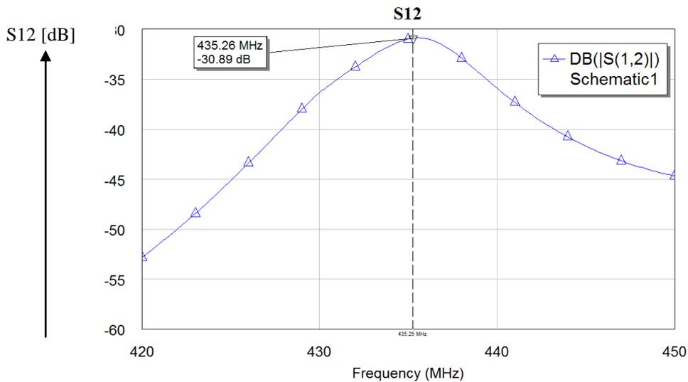
**Figure 2.27 :** The power amplifier's  $S_{12}$  graph.
