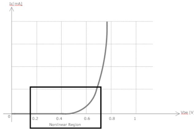
**Figure 2.32 :** Transistor’s nonlinear region.
