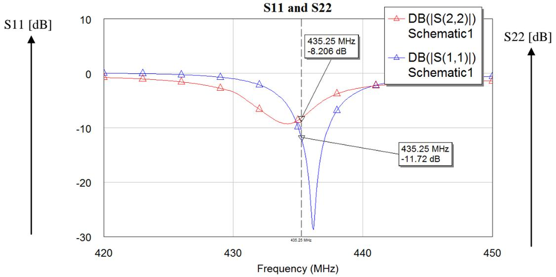
**Figure 2.26 :** The power amplifier's  $S_{11}$  and  $S_{22}$  graphs.
