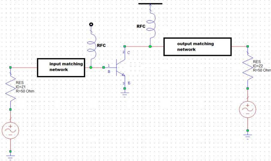
**Figure 2.53 :** The single-stage PA with matching circuits.
