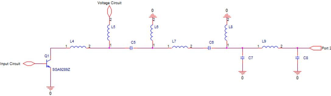
**Figure 2.55 :** The output matching circuit.
