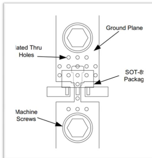
**Figure A.2 : Recommended mounting configuration.**
