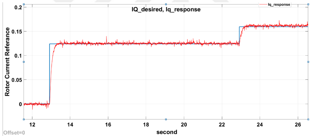
Figure 4.34 : Iq current characteristic at (-40) degree.
