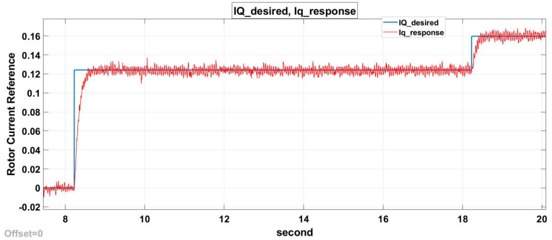
Figure 4.25 : Iq current characteristic at 25 kHz switching frequency.
