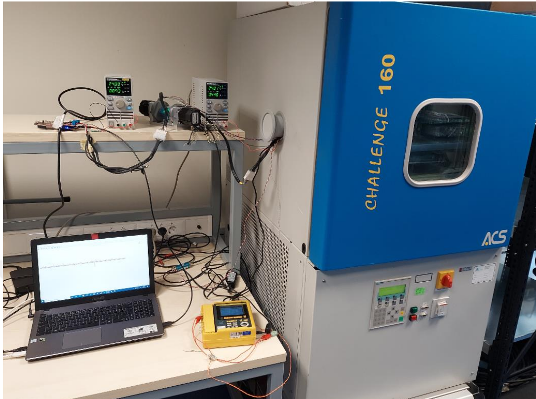
Figure 4.27 : Temperature test setup at the oven.
