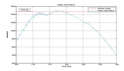
Figure 4.11: First Gear Acceleration Mass Estimation Results
