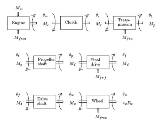
Figure 3.1: Powertrain Subsystems [14]
