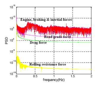
Figure 1.2: Comparison of Longitudinal Force Spectral Densities [2]
