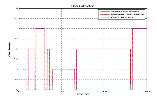
Figure 4.16: Gear Estimation Results
