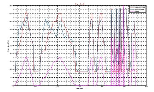
Figure 4.5: Neutral Gear Engine Speed
