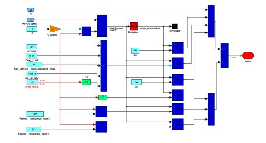
Figure 4.8: Mass Estimation Simulink Diagram
