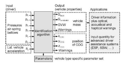
Figure 1.3: Payload Parameter Identification [7]
