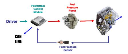
Figure 4.1: Engine System CAN Line
