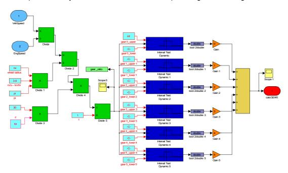
Figure 4.13: Initial Gear Estimation Algorithm Simulink Block
