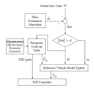
Figure 1.6: Overview of the Enhanced ESP system [15]
