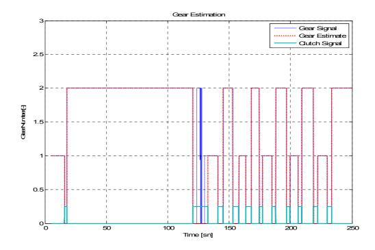
Figure 4.17: Gear Estimation Results
