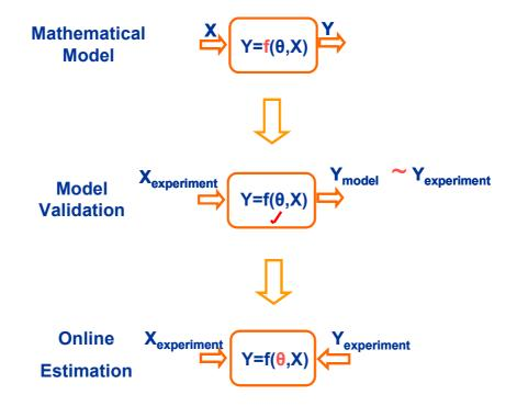
Figure 3.2: Model Based Estimation Process [18]
