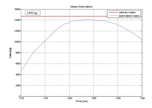
Figure 4.12: Low Pass Filtered Mass Estimation Results
