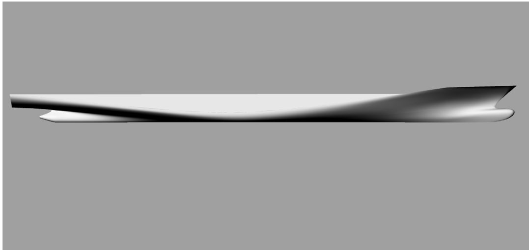
Figure 5.7 450m length form of container ship scaled by Rhino
