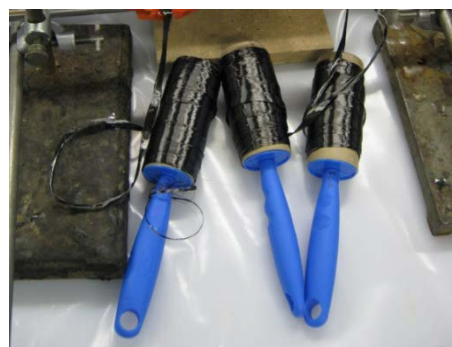
Figure 7.3 Dry/Hand lay-up fiber bundles using carbon fiber rolls.
