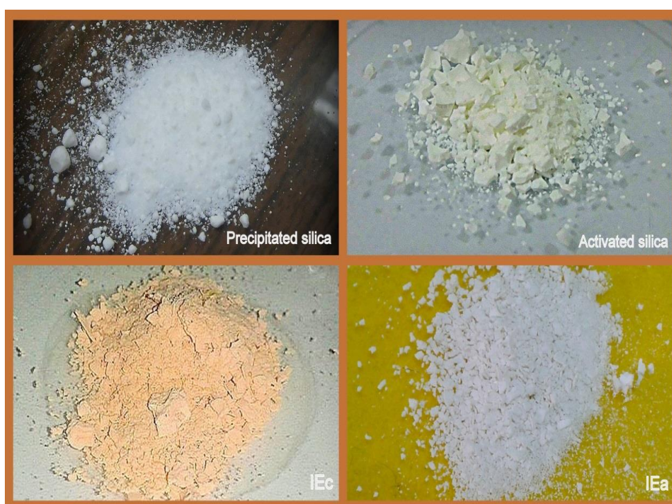
Figure 4.1 : CALB immobilization steps on precipitated silica.
