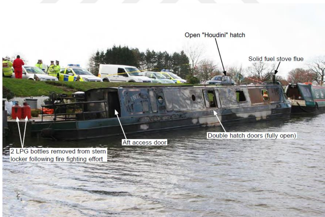
Figure 5.6 : View of Lindy Lou while fire investigation.
