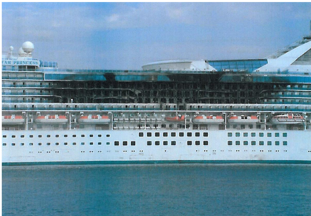
Figure 5.1 : View of Star Princess after fire incident.
