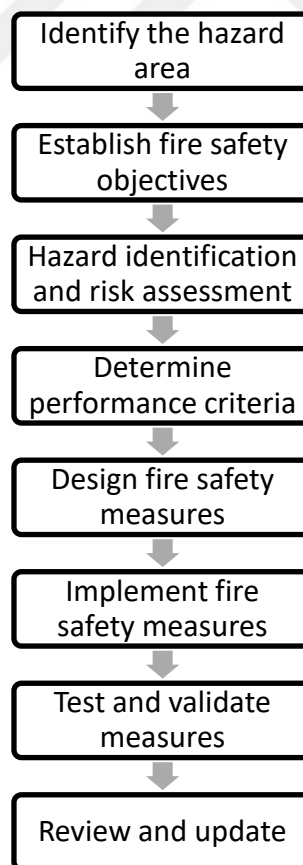
Figure 3.3 : Fire safety design steps (Rasbash et al, 2004).
