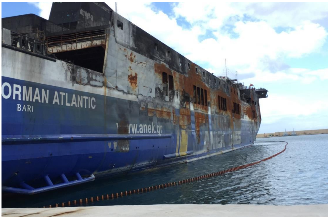
Figure 5.8 : View of Norman Atlantic after fire incident.
