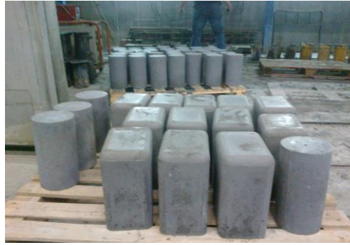
Figure 4.3: All Specimens after Taking Moulds
