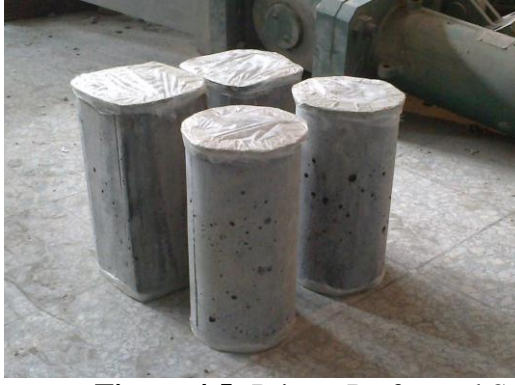
Figure 4.5: Primer Performed Specimens before Confining
