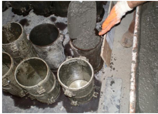
Figure 3.1: Casting the Specimens for Comparison
