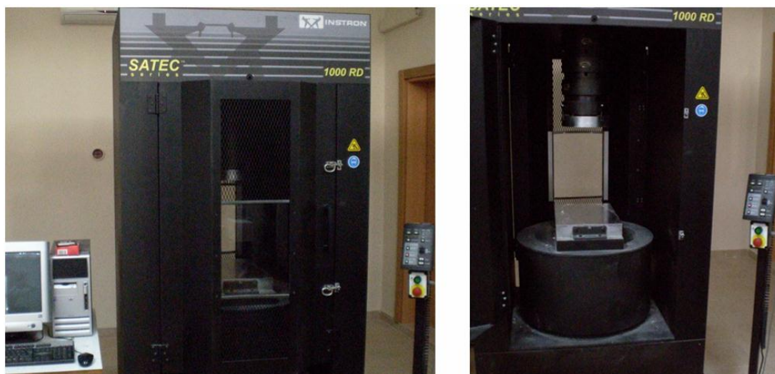
Figure 4.8 : 5000 kN Capacity Instron Test Machine
