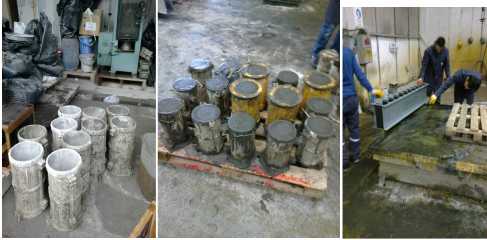
Figure 4.2: Moulds at Casting Step
