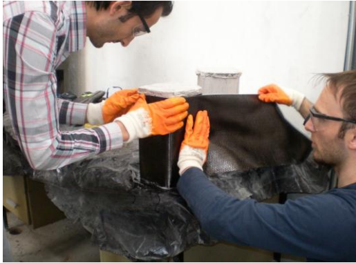
Figure 4.6: Confining the Specimens
