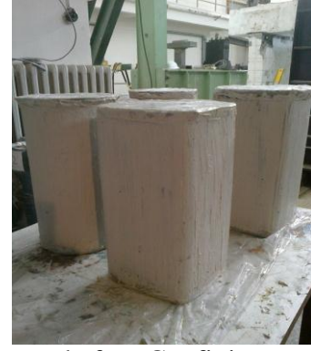
Figure 4.5: Primer Performed Specimens before Confining
