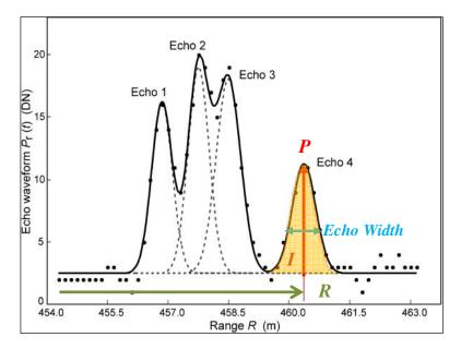
Figure 4.4 : Gaussian waveform decomposition (Wagner et al., 2008a).
