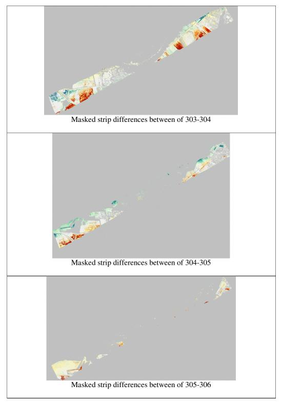
Figure E.1 (continued) : Height difference between overlapping strips.
