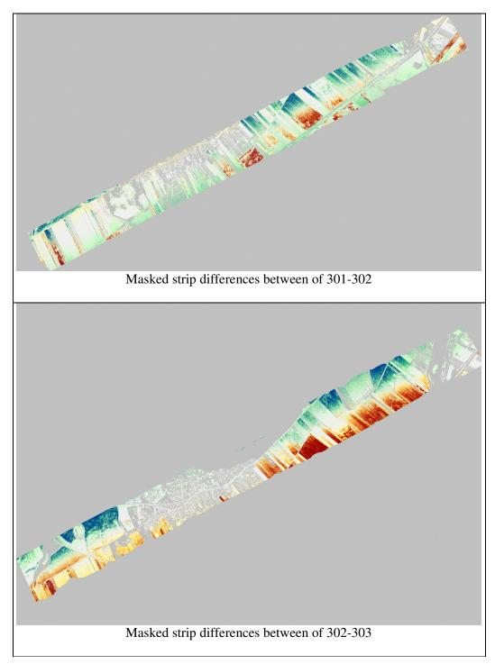
Figure E.1 : Height difference between overlapping strips.
