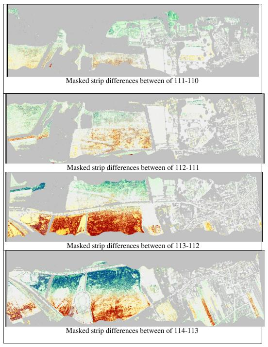
Figure E.1 (continued) : Height difference between overlapping strips.
