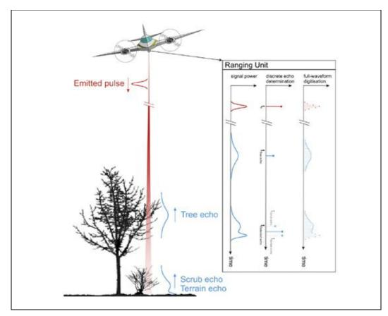
Figure 2.6 : Received echoe in FWF and discrete system (Doneus et al., 2008).
