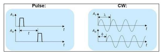
Figure 2.4 : Pulse (left) and CW (right) systems (Brenner, 2006).
