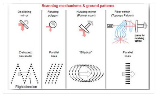
Figure 2.3 : General outlook to scanning mechanism (Brenner, 2006).
