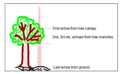
Figure 2.5 : Laser beam interaction with targets (Baltsavias, 2009).
