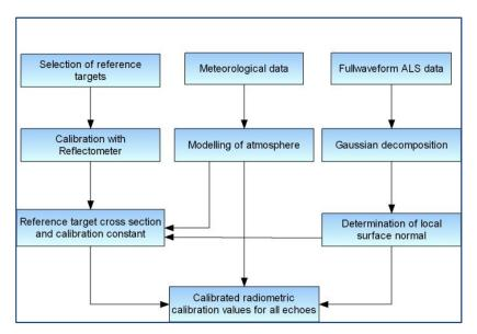
Figure 4.6 : Workflow of radiometric calibration.
