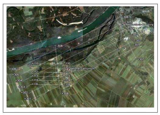
Figure 3.2 : Strips of ALS campaign from flight plan of Carnutnum (Airborne Technologies data sheet).
