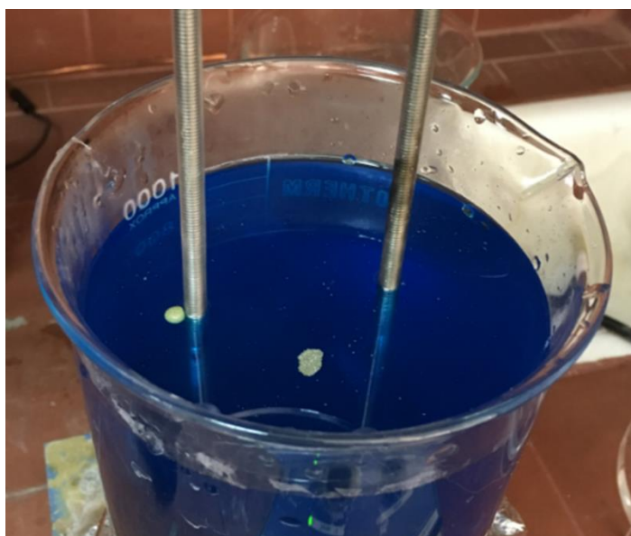
Figure 3.6 : Diamond particle clusters floating on the electrolyte surface.
