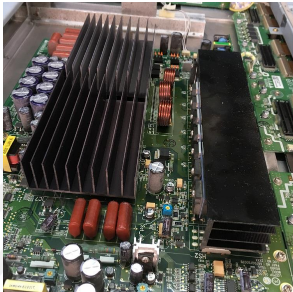
Figure 2.1 : Heat sink attached on a circuit board.
