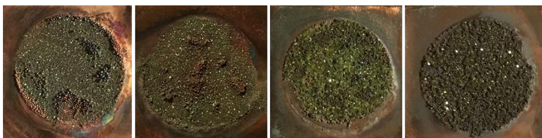
Figure 3.8 : First set of samples formed by using wet diamond particles.
