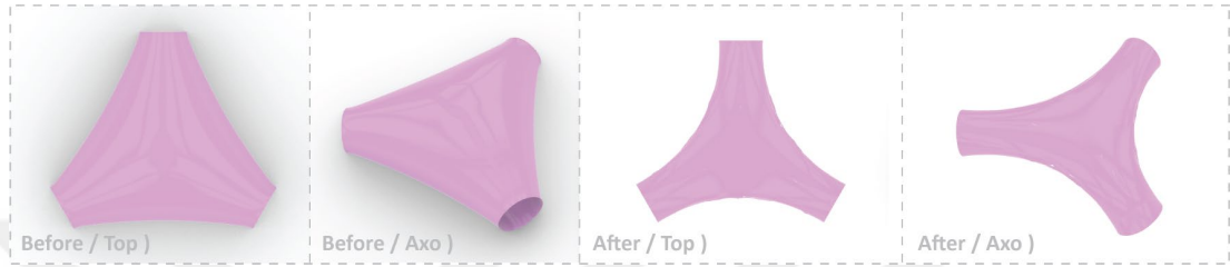
Figure 5.6 : A soap bubble film simulation was used for topology optimization of the structural element (Cilesizoglu et al., 2025).
