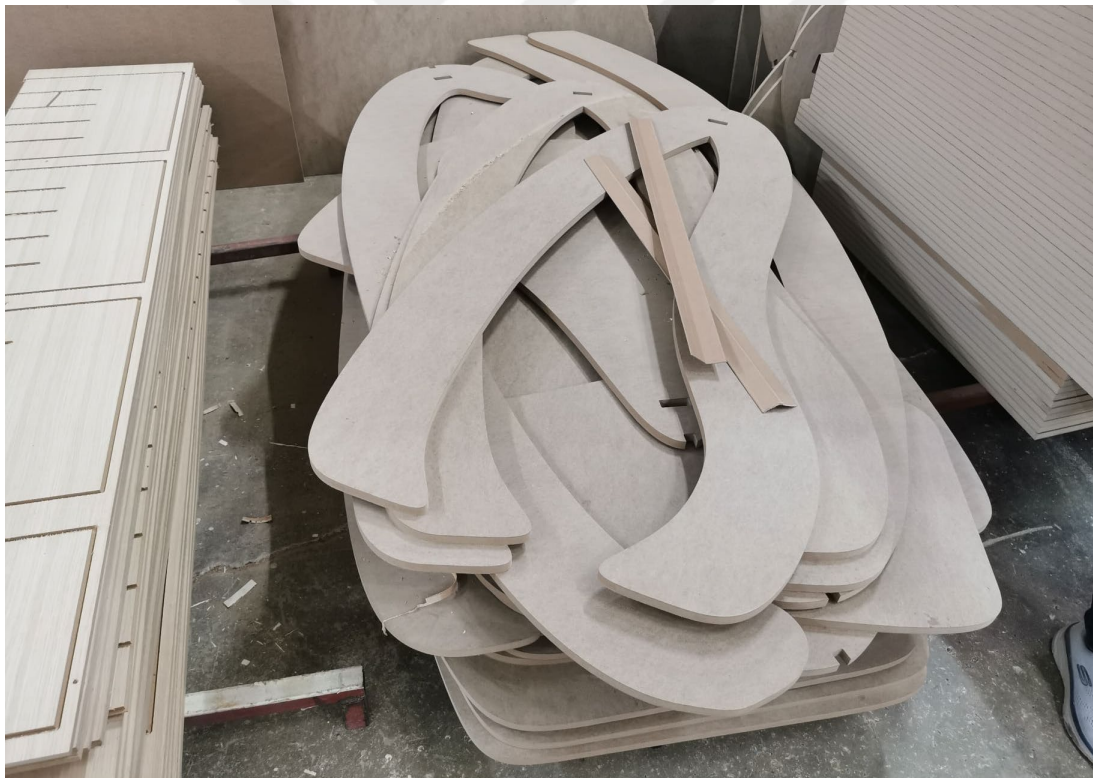
Figure 5.19 : CNC cut MDF panels (Cilesizoglu, 2024)
