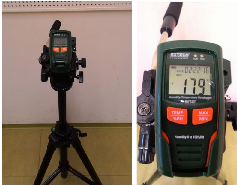
Figure 5.17 : RHT20 humidity and temperature data logger.
