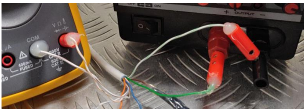
Figure A.2 : Connection order of vacuum gauge to power supply and multimeter.
