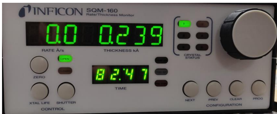
Figure A.3 : SQM160 thickness monitor.
