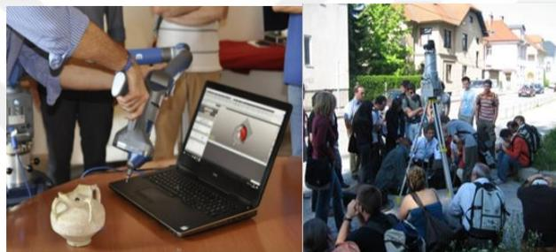
**Figure 2.2 :** Left: Scanning alcove with Faro laser arm application in the archeological museum, Right: demonstration of data acquisition with a Riegl brand ToF scanner.
