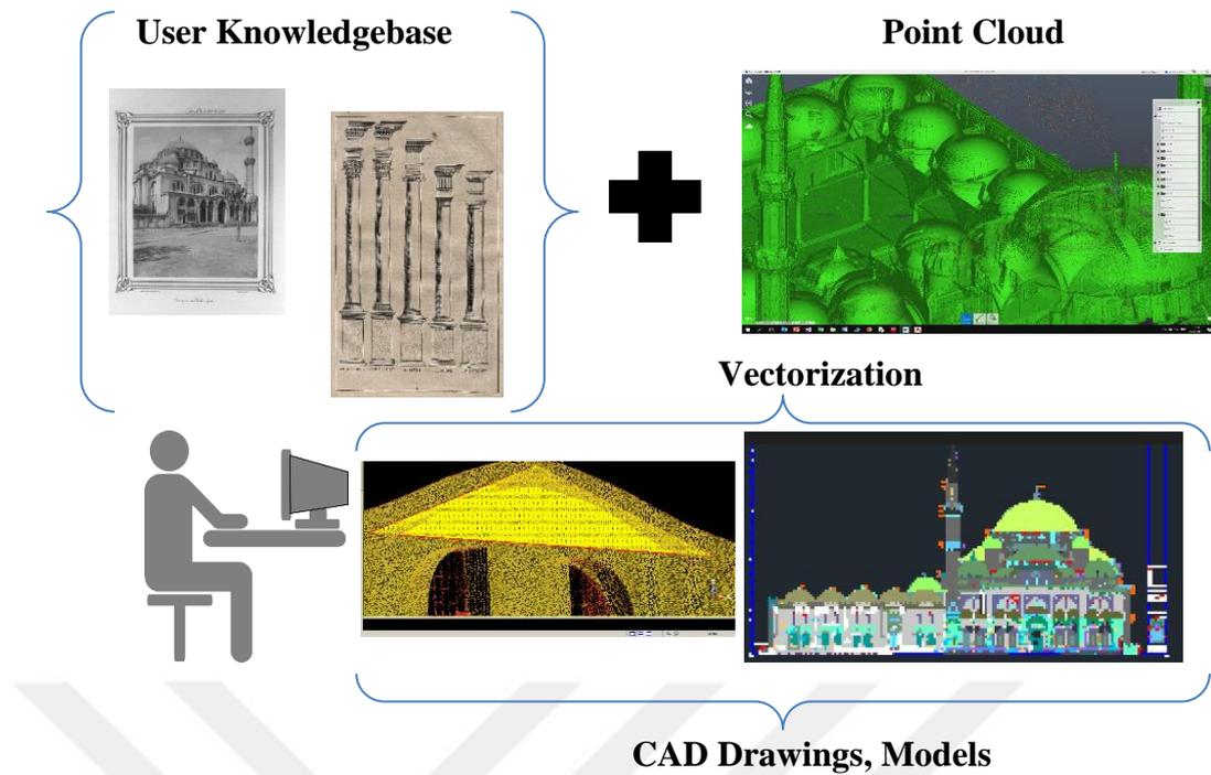
**Figure 2.4 :** Diagram depicting the process of conventional workflow from point cloud to products.
