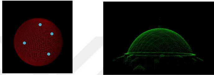
**Figure 4.11** : Left: Four non-coplanar points define a sphere in  $\mathbb{R}^3$ , right: example of the spherical dome in the point cloud.
