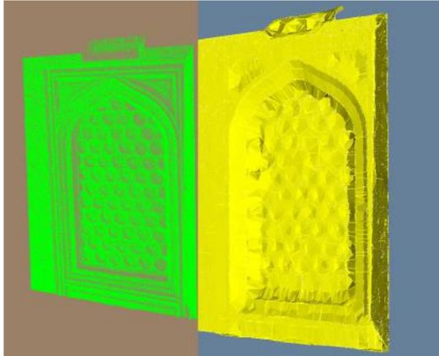
**Figure 2.7 :** Sample of a point cloud and implimenton of surface mesh based on Delanuay triangulation.
