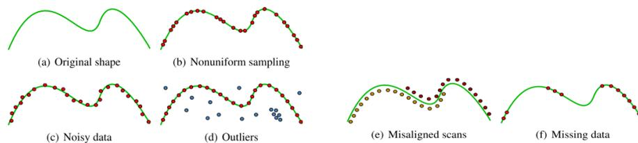
**Figure 2.5 :** Point cloud approximation issues to the real object as demonstrated as a curve in 2D (Berger et al., 2014).
