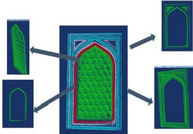
**Figure 5.6 :** Segmentation result of a complex arch window element.
