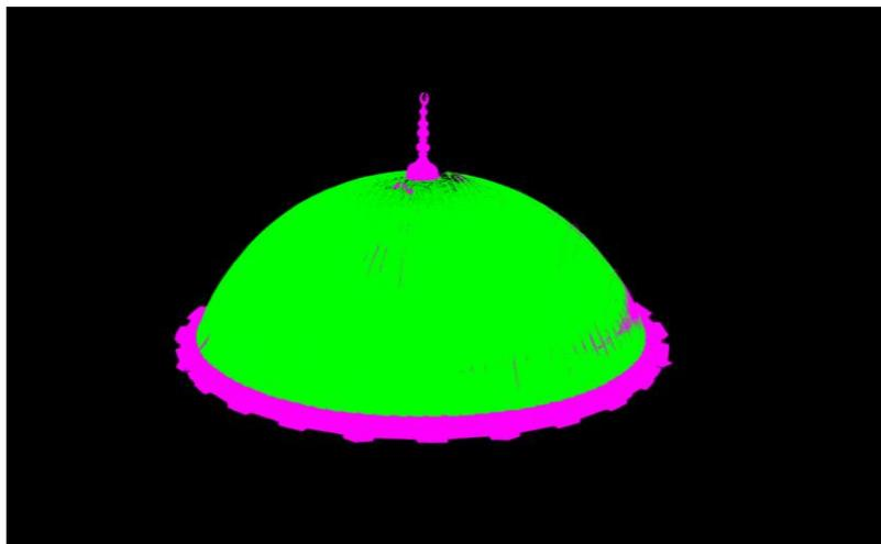
**Figure 5.9 :** Segmented point cloud of the outside dome.
