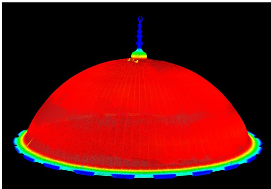
**Figure 6.1** : The distance of each point to the extracted parametric dome. Red color indicates the closest, and blue the furthest points.
