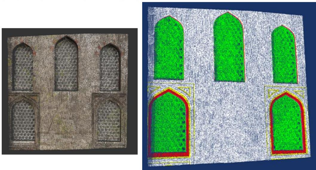
**Figure 5.7 :** Input point cloud of a window group and result of the segmentation.
