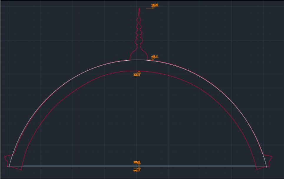
**Figure 6.2 :** Comparison of the Overlay of extracted Southeast Façade cross-section of the main dome (red) and the dome defined from the parameters from of methodology (white).
