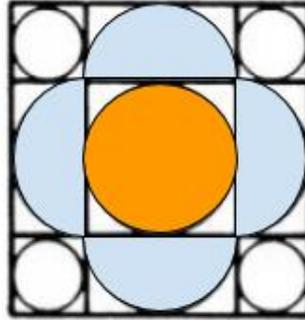
**Figure 4.5. :** Conceptual variations of semi-dome layout in Sinan's designs adapted from Kuban, (1987).
