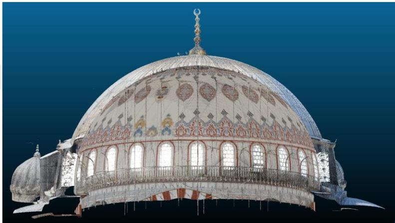
**Figure 5.8 :** Top: Dome view of the point cloud. Bottom: A cross section of the input point cloud, displaying both indoor and outside of the main dome.
