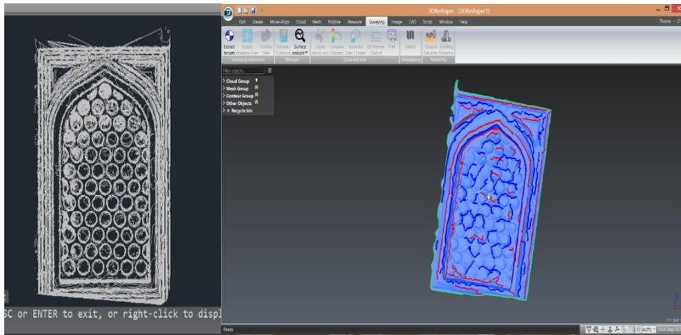
**Figure 2.6 :** Our experiment with Leica Cyclone and 3D reshaper software with automatic feature extracting algorithms.
