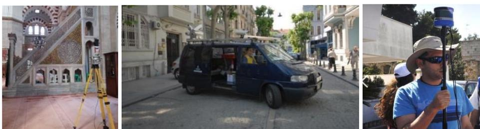
**Figure 2.3 :** Use of TLS scanners in static (left), mobile (middle), and handheld.
