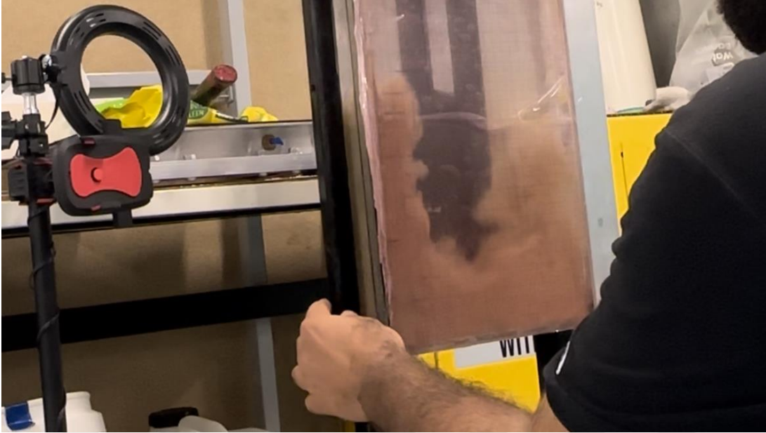
Figure 3.6 : Tilting box experiments to fathom critical angle slope.
