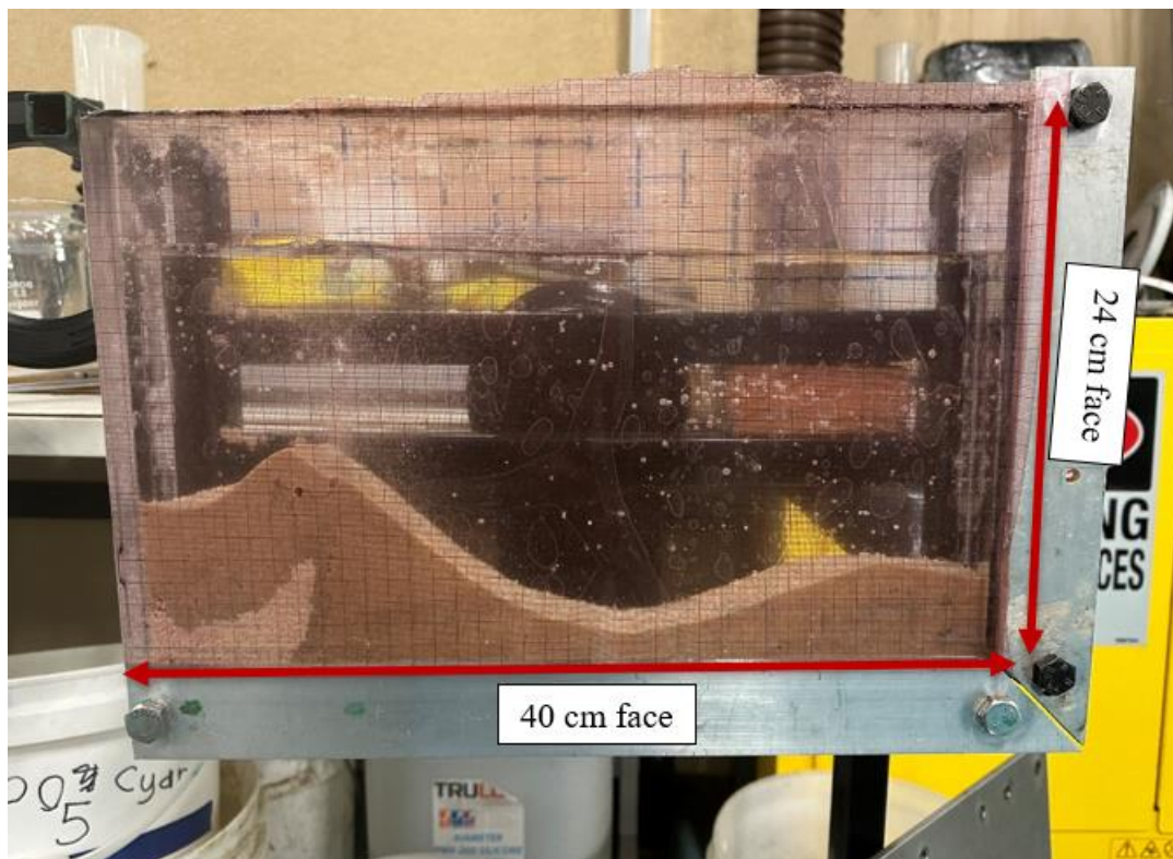
Figure 3.4: Tilting box experiments under different scenarios of sand, fluids, and tilting speed.
