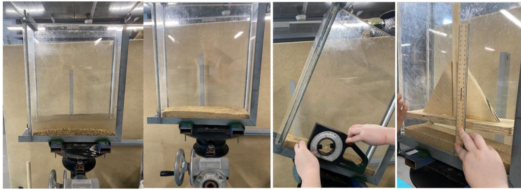
Figure 3.7 : Friction angle determination for different sort of sand.
