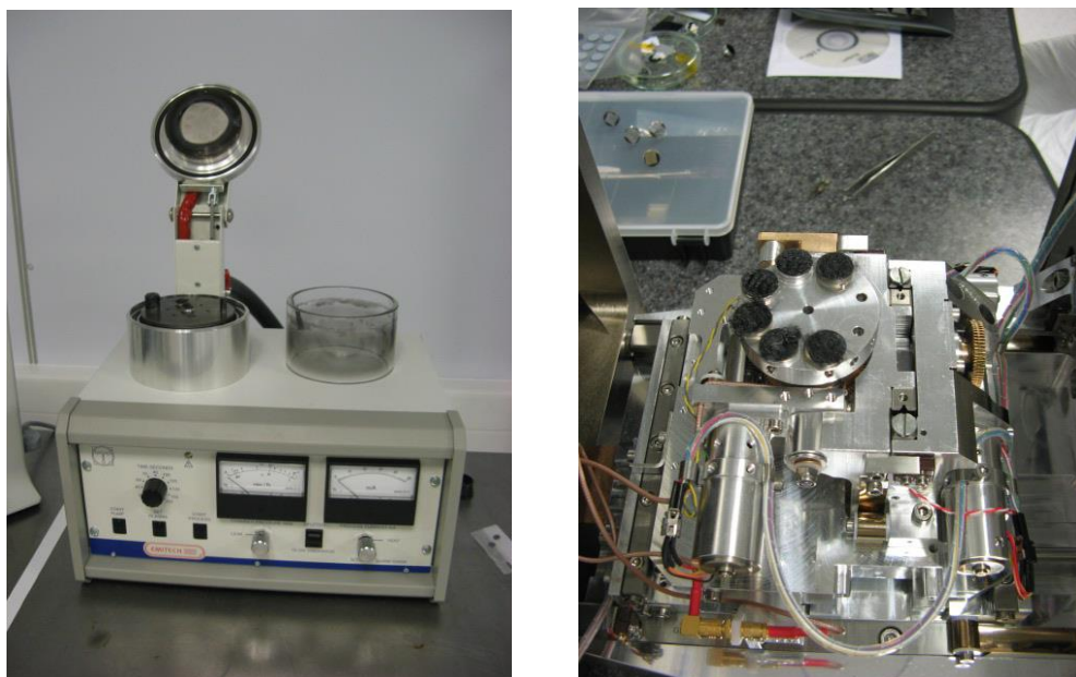
Figure 4.8 : Film coating by Emitech sputter coater and preparation of specimens.
