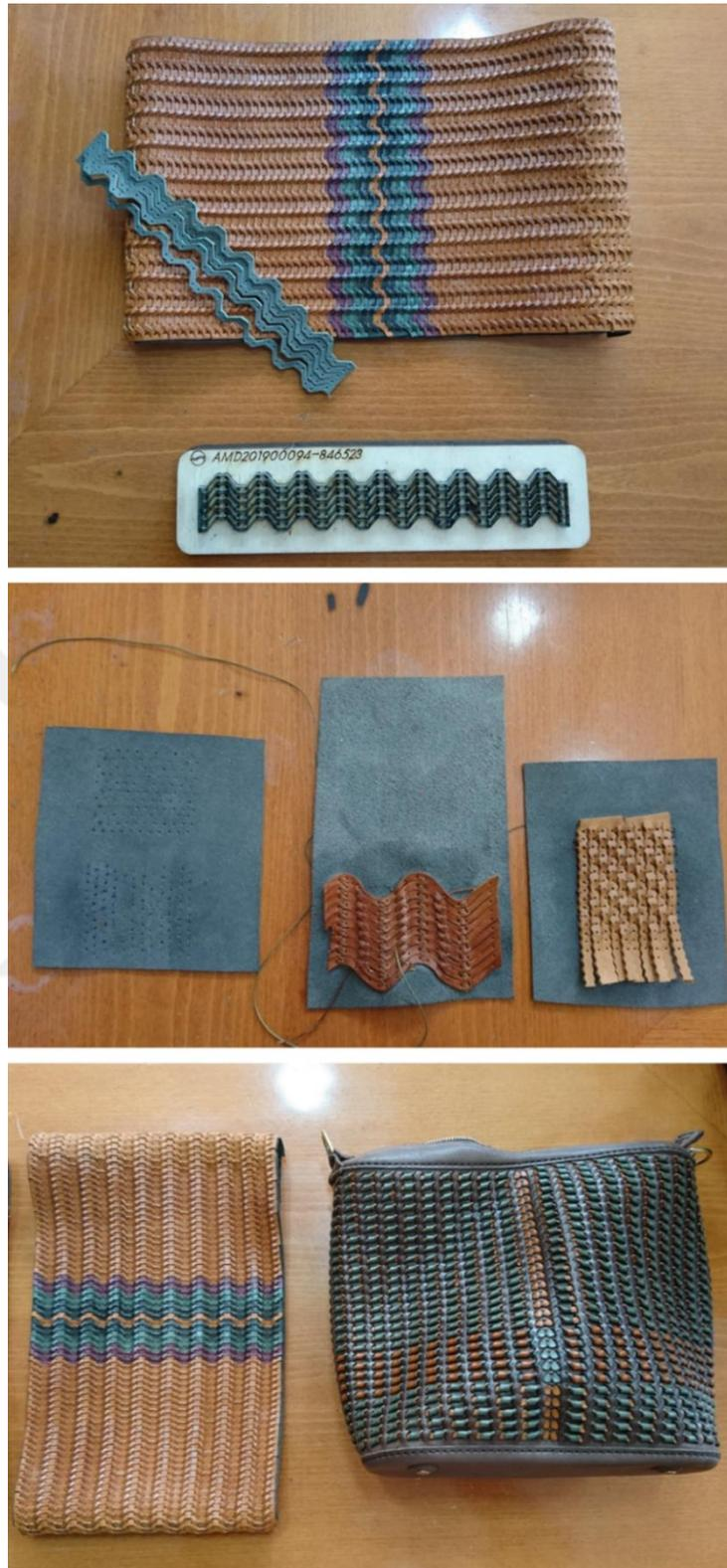
**Figure 6.21 :** Mould, pattern of handmade bags and final product, Company E.
