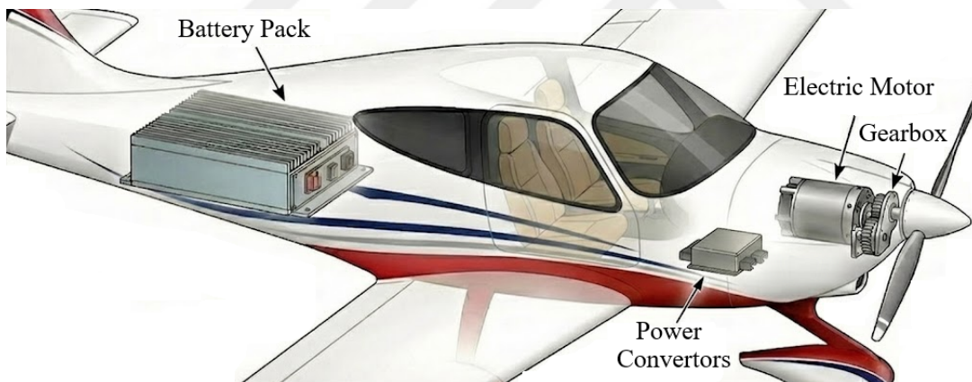
Figure 4.3: Schematic modeling of the Tecnam P2008 JC Aircraft's all-electric propulsion system.
