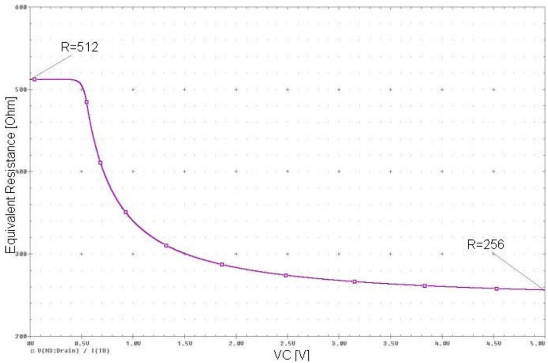
**Figure 2.4:** The change of the total equivalent resistance of the parallel triode MOSFETs.
