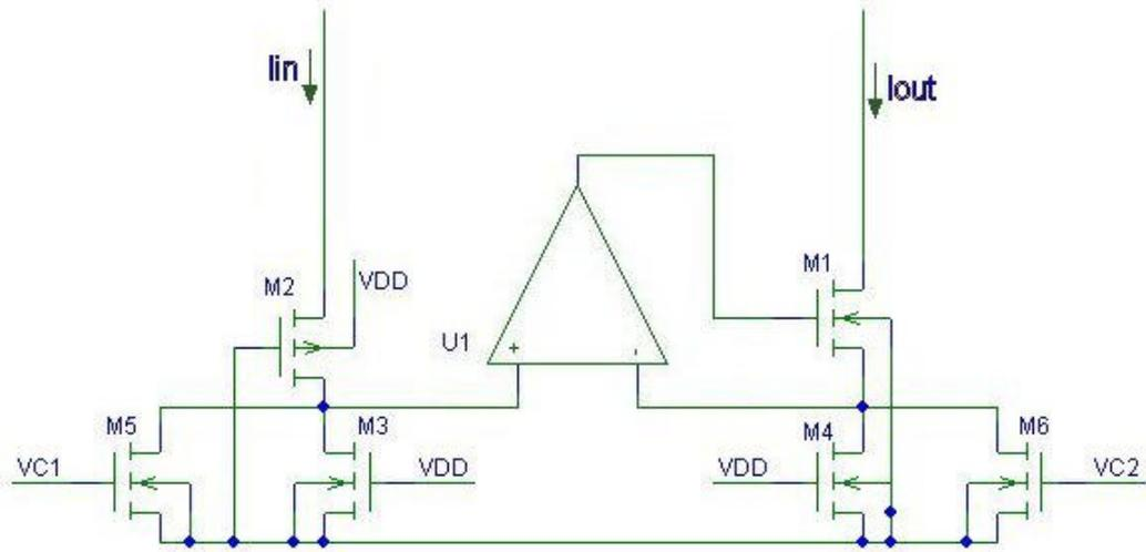
**Figure 2.1:** The conceptual circuit schematic of the tunable current mirror with triode MOSFETs.
