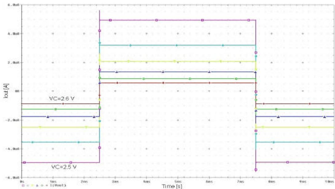
**Figure 2.51:** Pulse response of the tunable current mirror with current dividers in the compensated situation.
