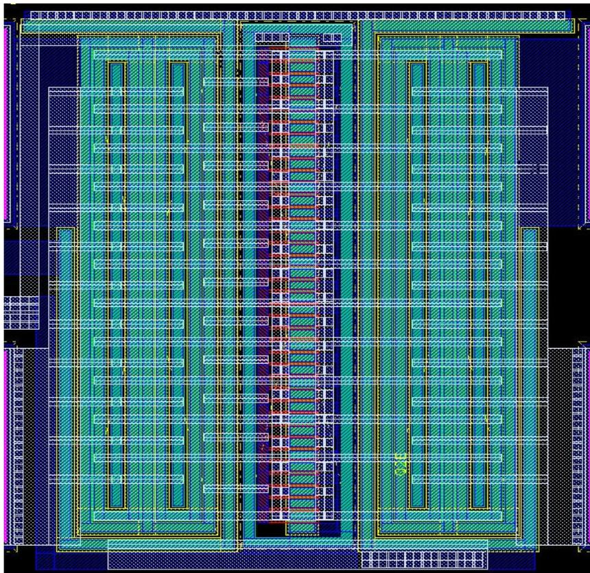
**Figure 2.63:** Layout of the core of the tunable current mirror with BJT differential pair topology.
