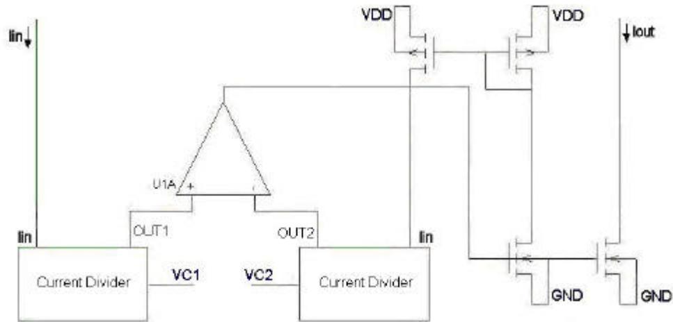
**Figure 2.37:** The conceptual schematic of the tunable current mirror with current dividers.
