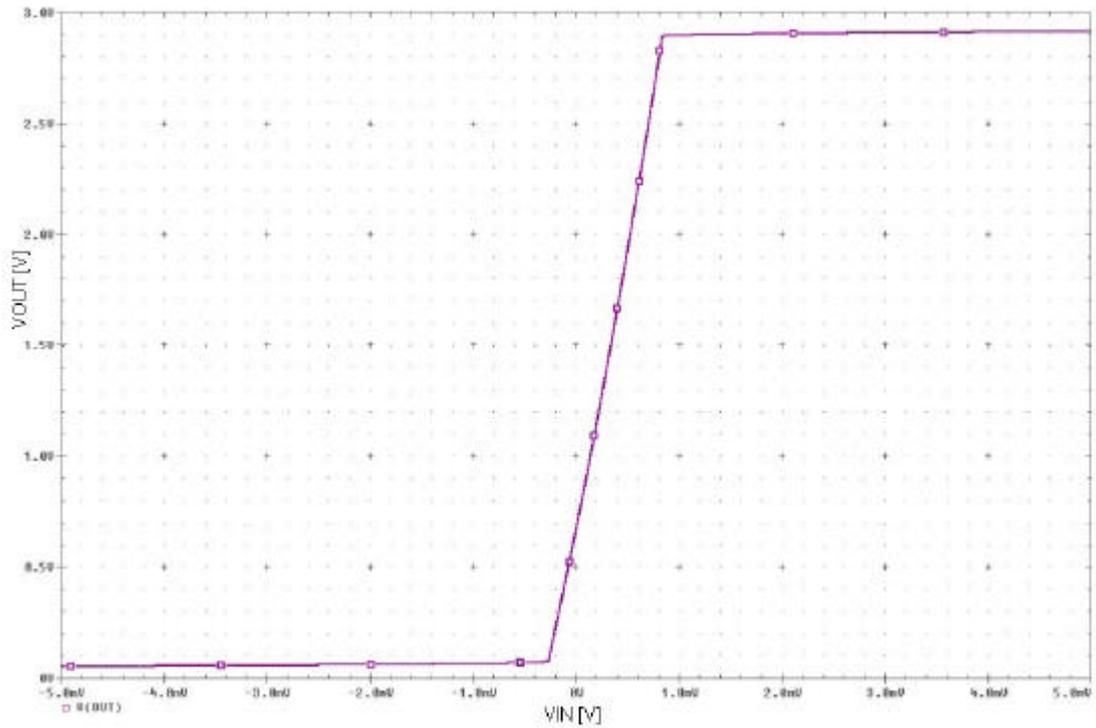
**Figure 2.9:** DC sweep simulation result of the opamp.
