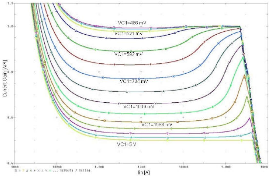
**Figure 2.11:** The change of the gain of the tunable current mirror with triode MOSFETs for different  $V_{C1}$  values.
