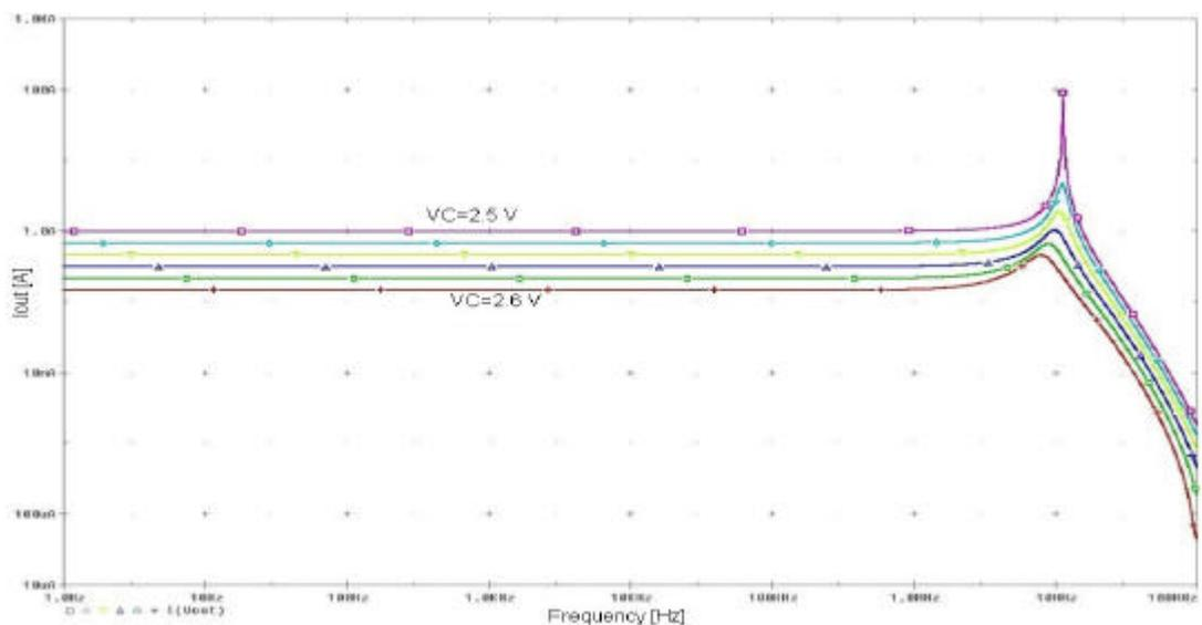
**Figure 2.47:** AC response of the tunable current mirror with current dividers when the gain is greater than unity.
