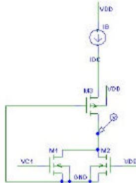
**Figure 2.3:** The schematic used for the simulation of the change of total equivalent resistance of the parallel triode MOSFETs.
