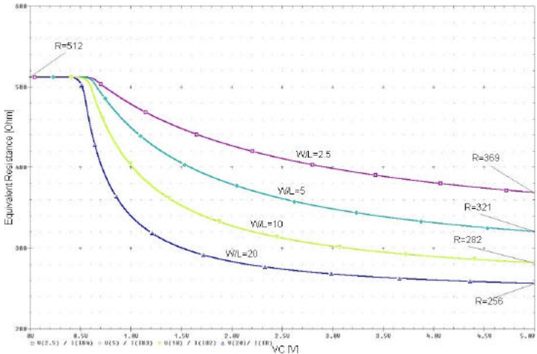
**Figure 2.5:** Affect of the W/L ratio of the controlled triode MOSFET over the total equivalent resistance.
