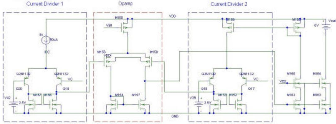
**Figure 2.42:** Circuit schematic of the tunable current mirror with current dividers.
