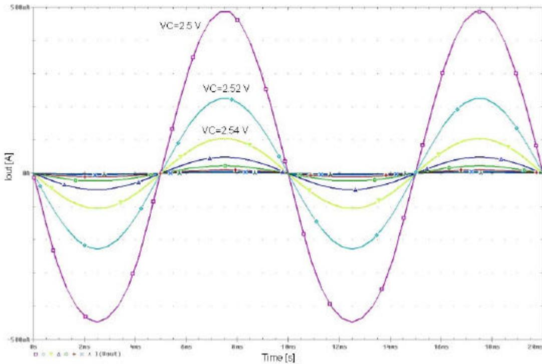
**Figure 2.44:** Transient simulation result of the tunable current mirror with current dividers when the gain is smaller than unity.
