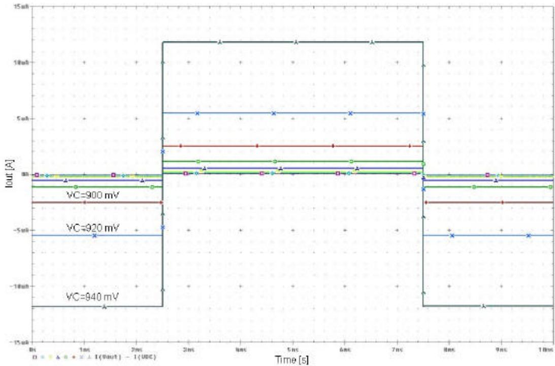
**Figure 2.60:** Pulse response of the tunable current mirror with BJT differential pair for the gains greater than unity.
