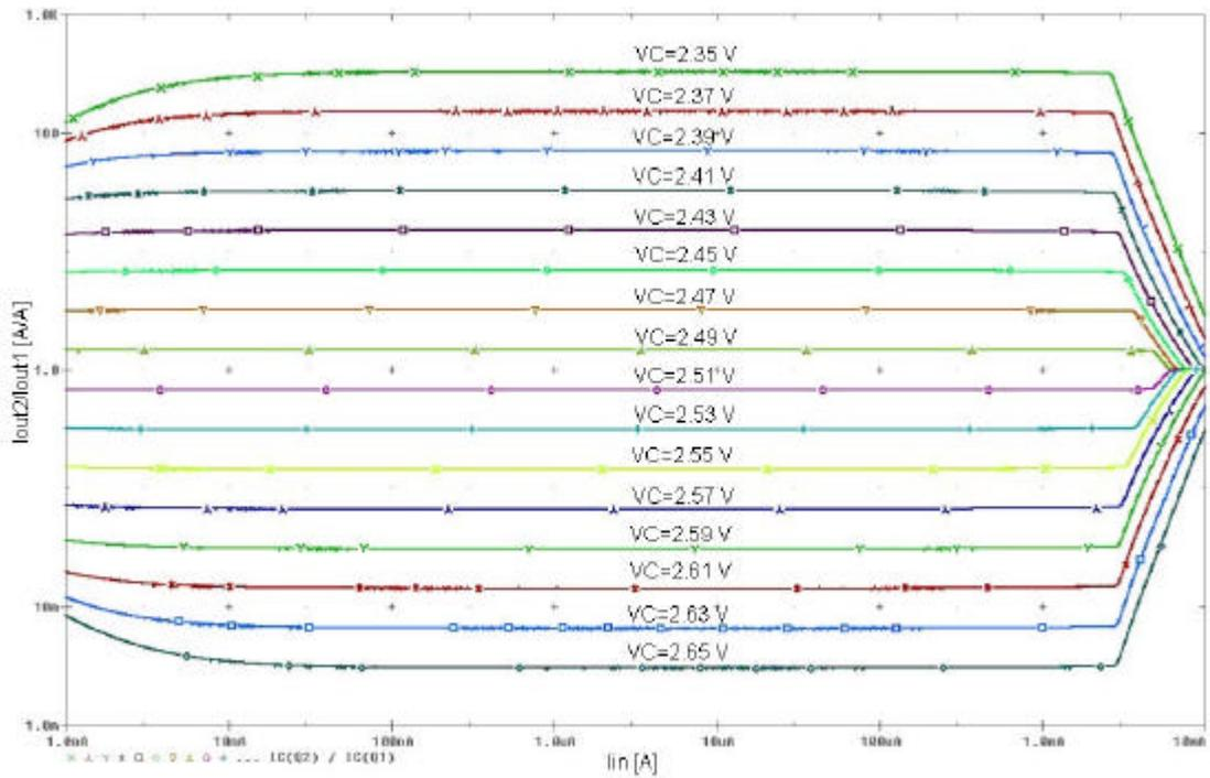
**Figure 2.41:** The change in the ratio between two output currents of the current divider for different values of  $V_C$ .
