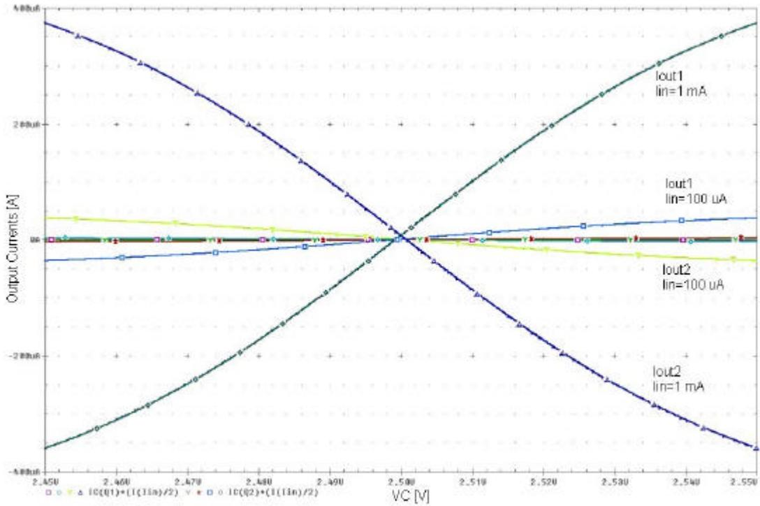
**Figure 2.40:** The transition characteristic of output currents of the current divider according to  $V_C$  for different values of input current (from 1  $\mu$ A to 1 mA with one decade steps).
