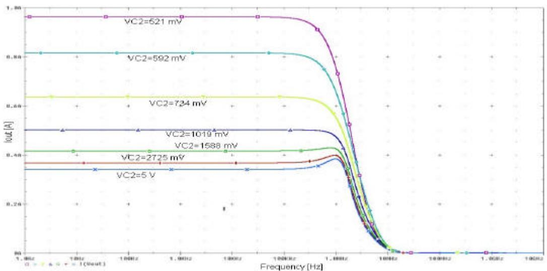
**Figure 2.31:** The AC simulation result of the tunable current mirror with VGAs obtained by changing  $V_{C2}$  in the compensated situation.
