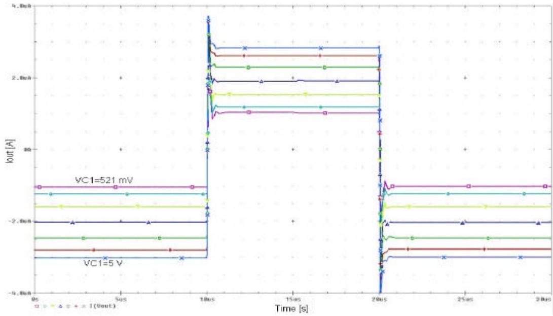
**Figure 2.34:** The pulse response of the tunable current mirror with VGAs for the uncompensated situation, obtained by changing  $V_{C1}$ .
