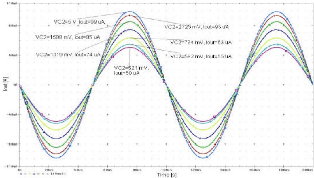
**Figure 2.16:** The result of the transient simulation run on the tunable current mirror with triode MOSFETs by changing  $V_{C2}$ .
