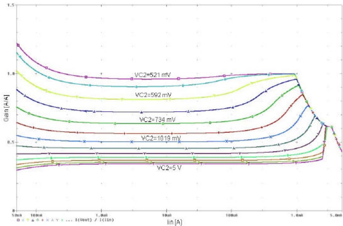
**Figure 2.27:** The change of the gain of the tunable current mirror with VGAs for different  $V_{C2}$  values.
