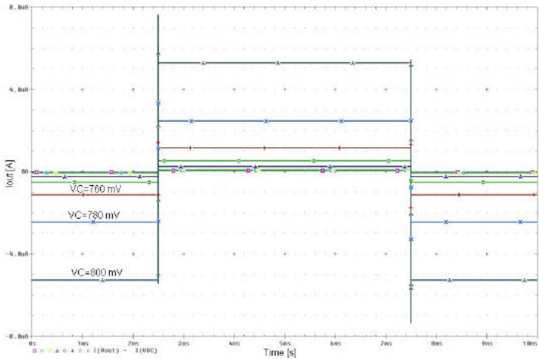
**Figure 2.61:** Pulse response of the tunable current mirror with BJT differential pair for the gains smaller than unity.
