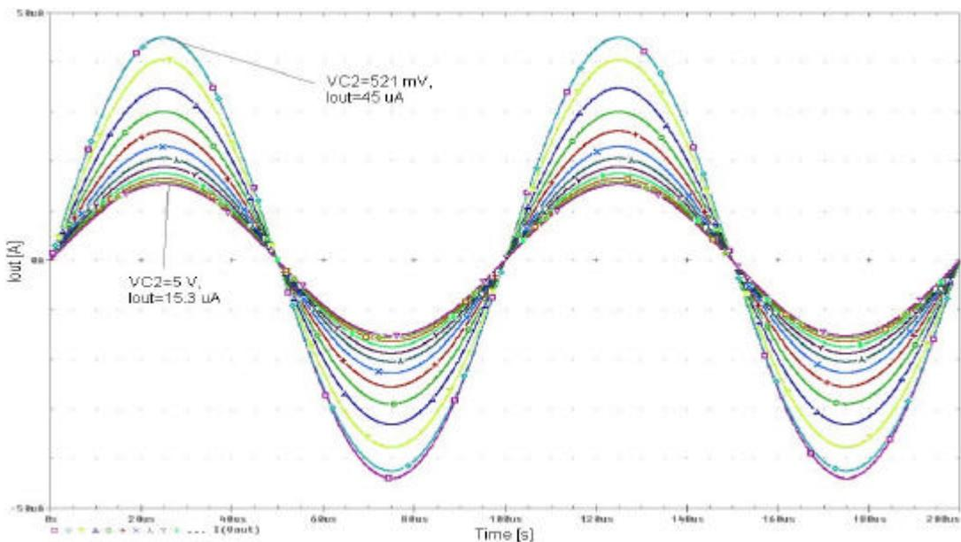
**Figure 2.33:** The transient simulation result of the tunable current mirror with VGAs obtained by changing  $V_{C2}$ .
