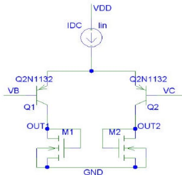
**Figure 2.38:** The circuit schematic of the current divider.
