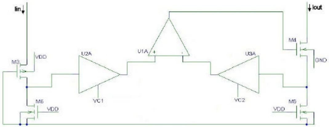
**Figure 2.20:** The conceptual schematic of the tunable current mirror with VGAs.
