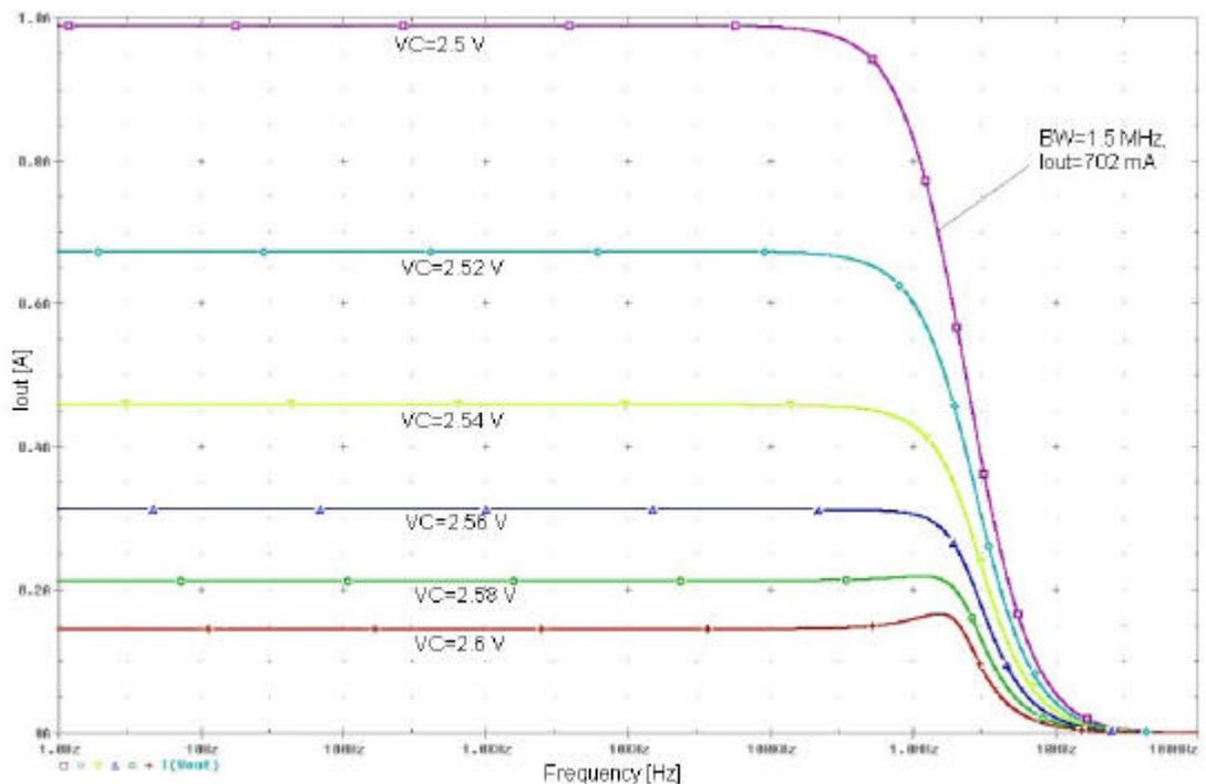
**Figure 2.49:** AC response of the tunable current mirror with current dividers in the compensated situation.
