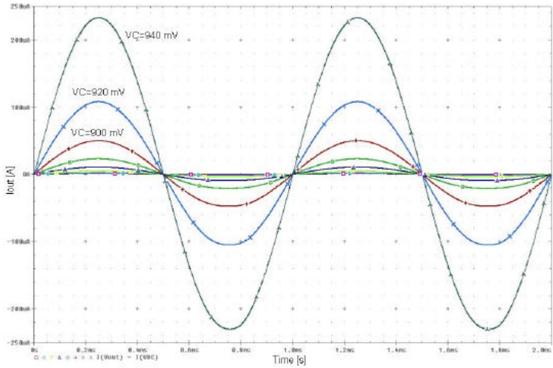
**Figure 2.58:** Transient simulation of the tunable current mirror with BJT differential pair with sinusoidal input for gains greater than unity.
