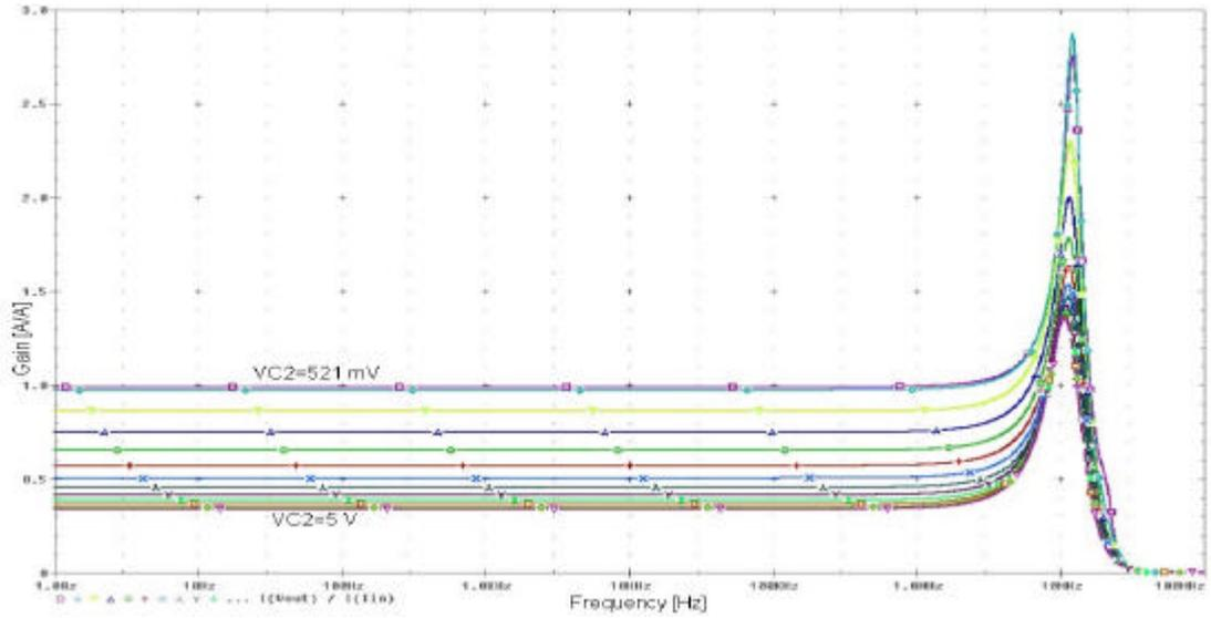
**Figure 2.30:** The AC simulation result of the tunable current mirror with VGAs obtained by changing  $V_{C2}$  in the uncompensated situation.
