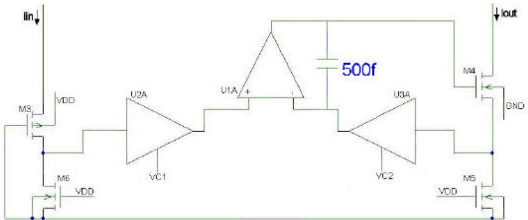
**Figure 2.28:** The compensation configuration of the tunable current mirror with VGAs.
