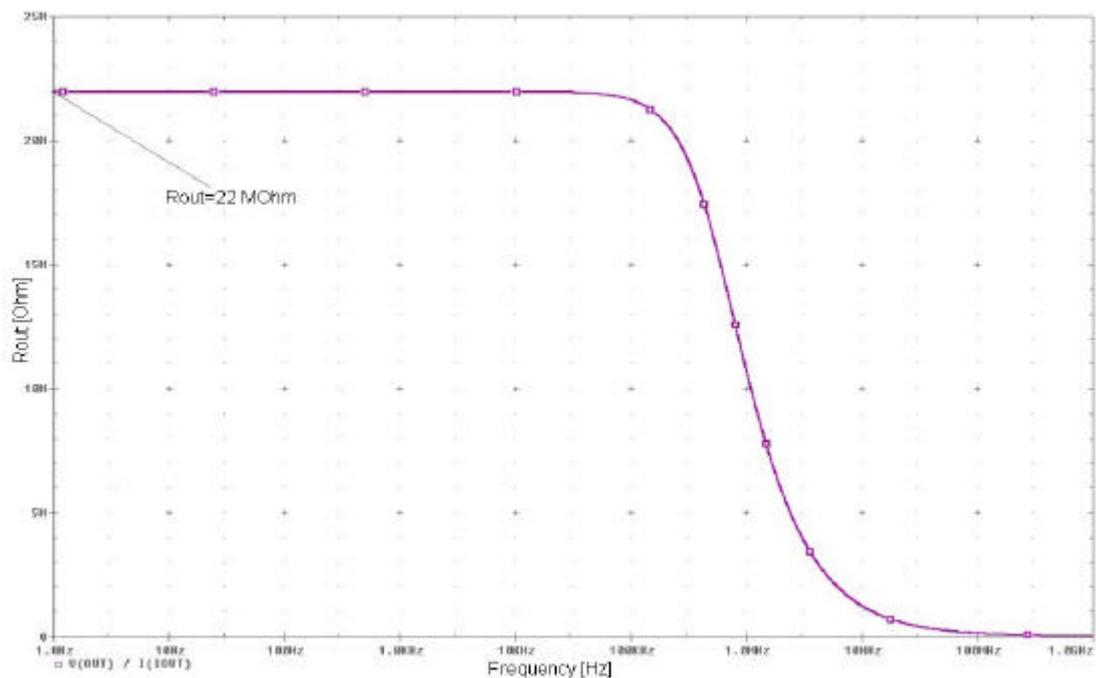
**Figure 2.10:** The output resistance of the opamp.
