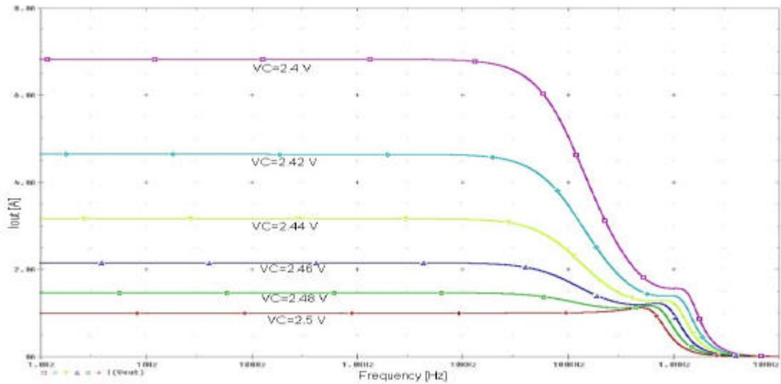
**Figure 2.46:** AC response of the tunable current mirror with current dividers when the gain is smaller than unity.
