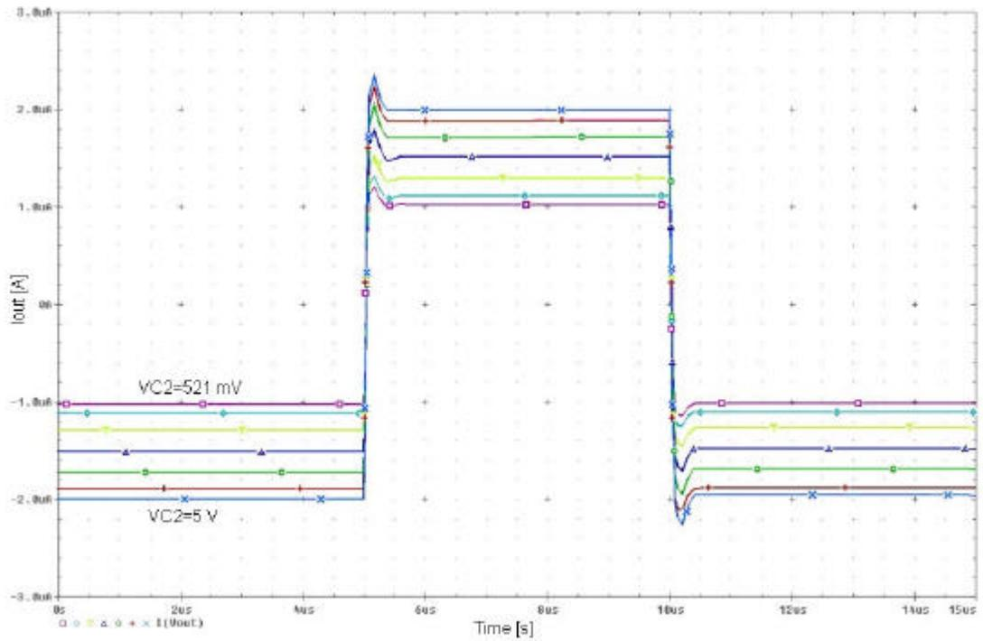
**Figure 2.19:** The pulse response graphics of the tunable current mirror with the triode MOSFETs obtained by changing  $V_{C2}$ .
