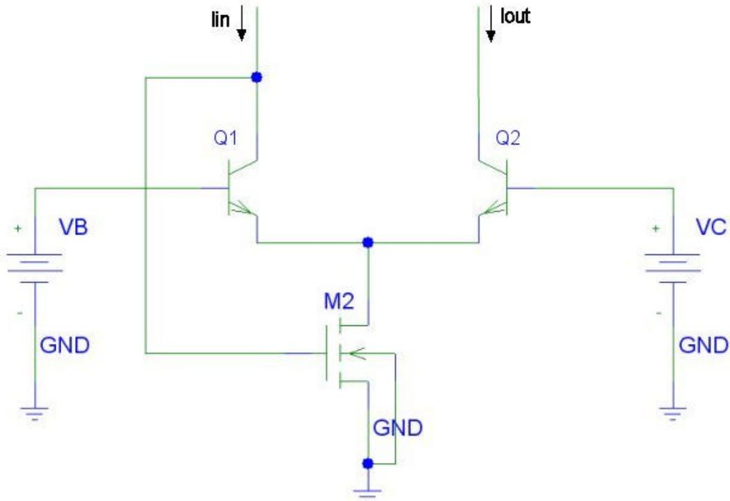
**Figure 2.54:** Schematic of tunable current mirror with BJT differential pair.
