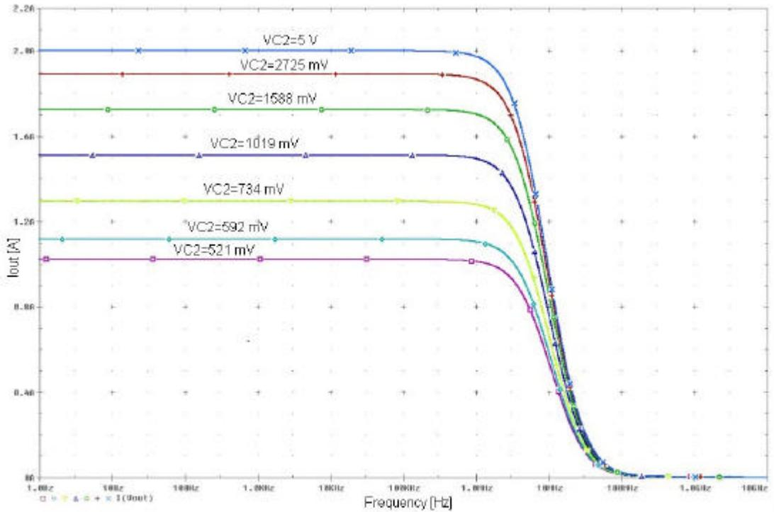
**Figure 2.14:** AC simulation result of the tunable current mirror with triode MOSFETs for different  $V_{C2}$  control voltage values.
