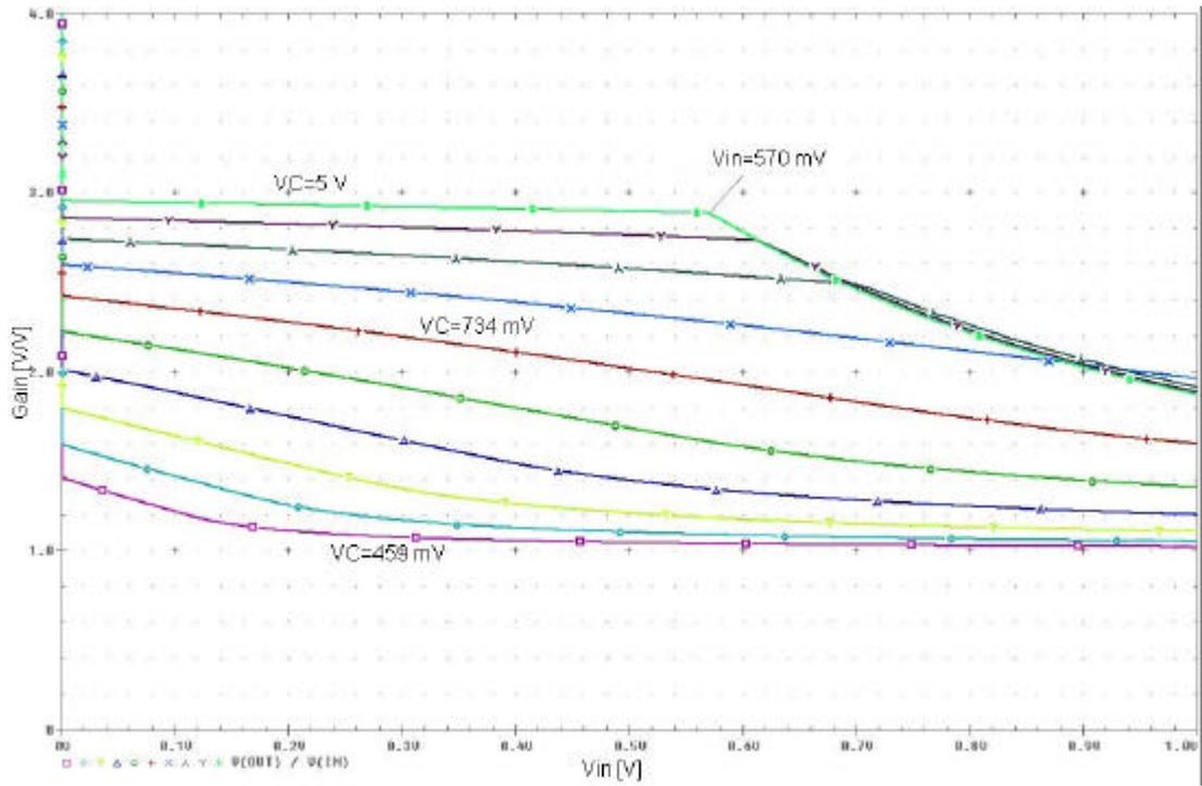
Figure 2.24: DC simulation result of the VGA circuit.
