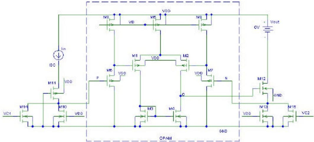
**Figure 2.2:** The realization of the tunable current mirror with triode MOSFETs.
