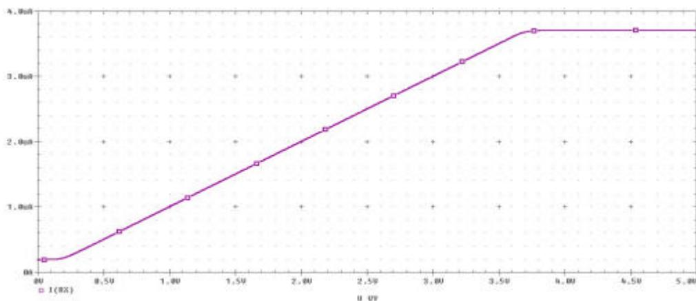
**Figure 2.65:**  $I_X$  current of ECCII for DC voltage sweep applied to Y.
