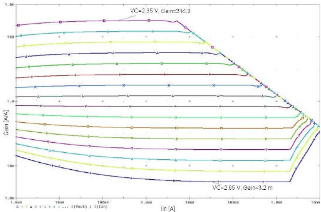
**Figure 2.43:** The change of the gain of the tunable current mirror with current dividers for different  $V_C$  values.
