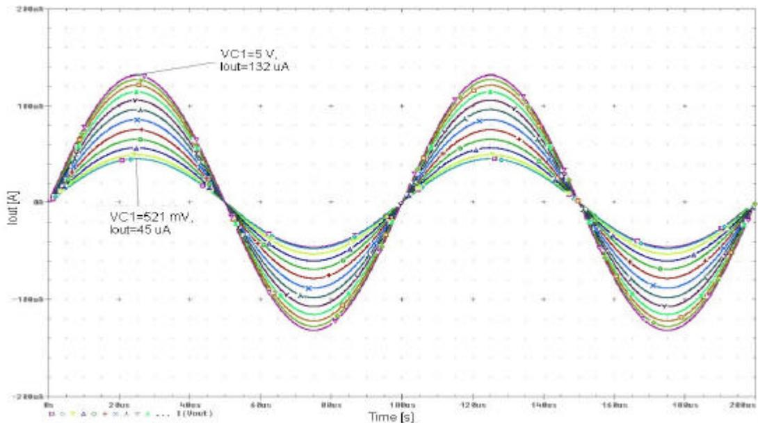
**Figure 2.32:** The transient simulation result of the tunable current mirror with VGAs obtained by changing  $V_{C1}$ .
