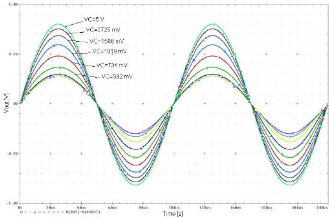
Figure 2.25: Transient simulation result of the VGA circuit.
