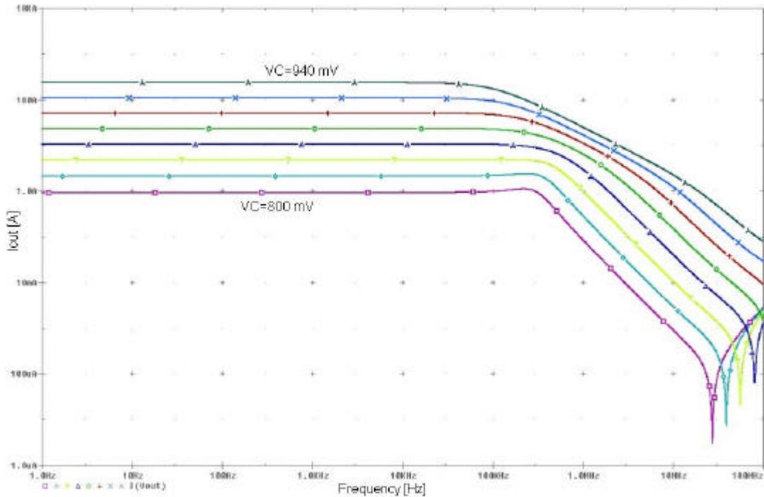
**Figure 2.57:** AC response of the tunable current mirror with BJT differential pair for high gain values.
