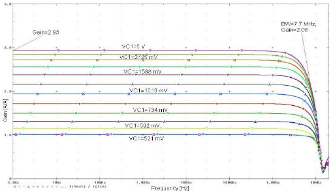
**Figure 2.29:** The AC simulation result of the tunable current mirror with VGAs obtained by changing  $V_{C1}$  in the uncompensated situation.
