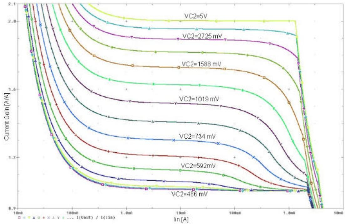
**Figure 2.12:** The change of the gain of the tunable current mirror with triode MOSFETs for different  $V_{C2}$  values.
