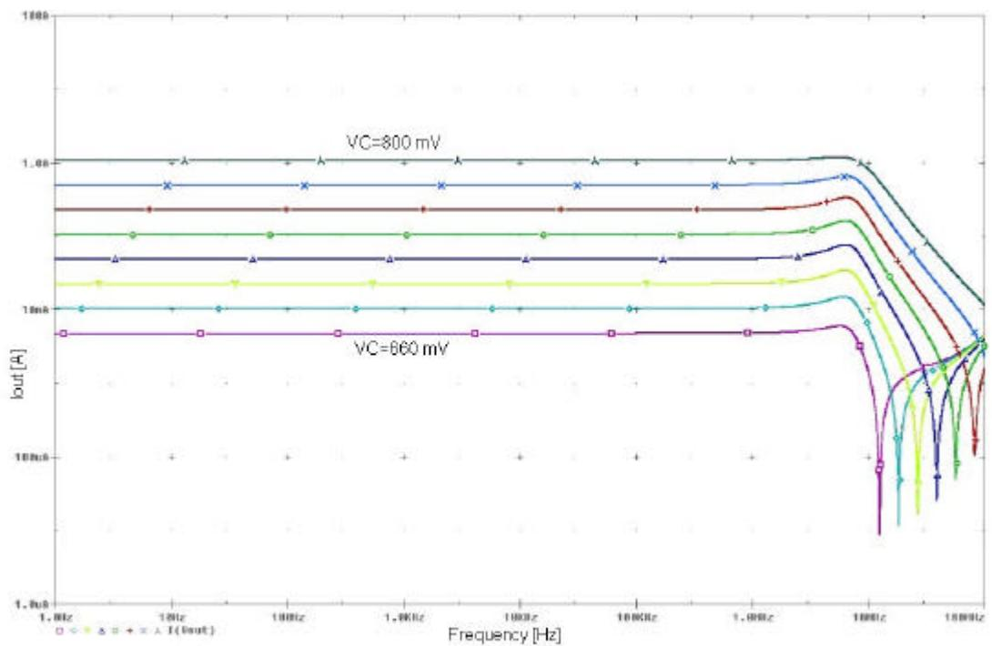
**Figure 2.56:** AC response of the tunable current mirror with BJT differential pair for low gain values.
