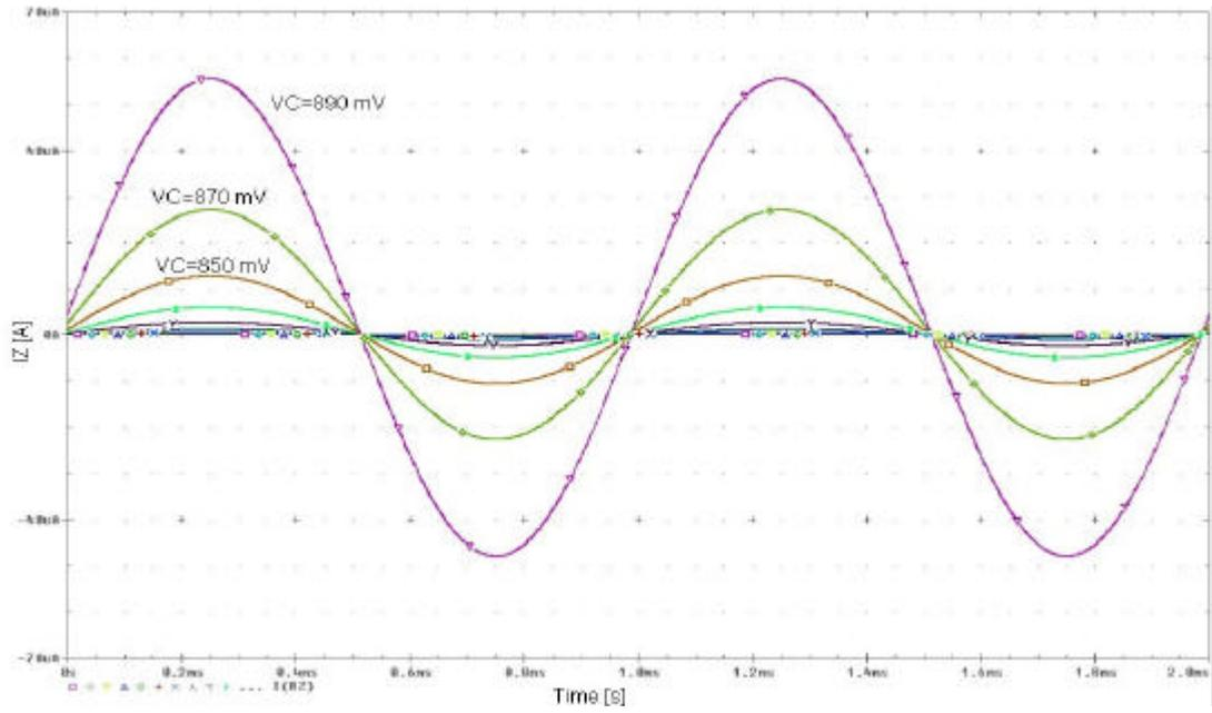
**Figure 2.69:**  $I_Z$  current of the ECCII for sinusoidal voltage source applied to Y.
