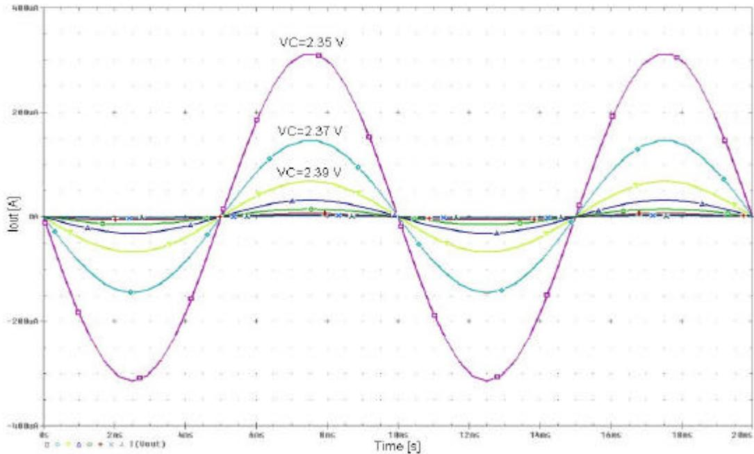
**Figure 2.45:** Transient simulation result of the tunable current mirror with current dividers when the gain is greater than unity.
