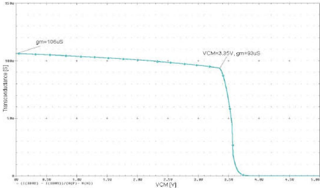
**Figure 2.8:** The change of the transconductance of the single stage opamp according to the input common mode voltage.
