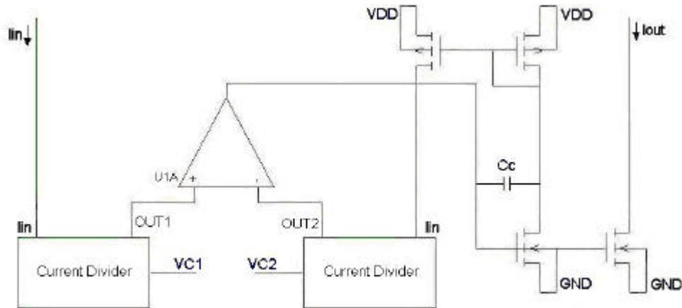
**Figure 2.48:** Compensation of the tunable current mirror with current dividers.
