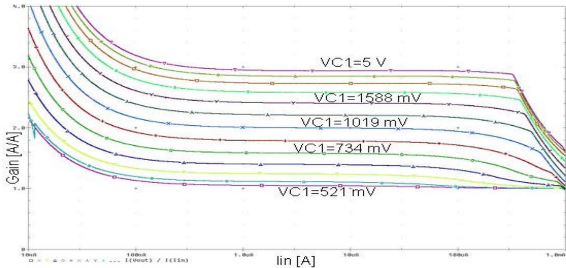
**Figure 2.26:** The change of the gain of the tunable current mirror with VGAs for different  $V_{C1}$  values.
