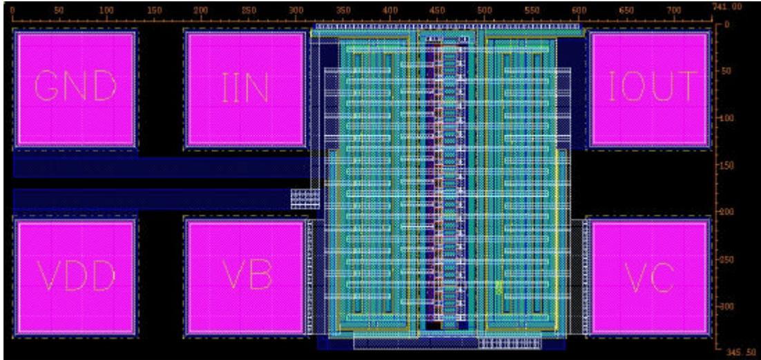
**Figure 2.62:** Layout of the tunable current mirror with BJT differential pair.
