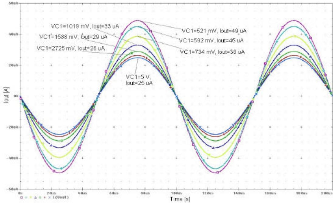
**Figure 2.15:** The result of the transient simulation run on the tunable current mirror with triode MOSFETs by changing  $V_{C1}$ .
