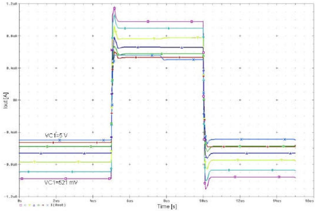
**Figure 2.18:** The pulse response graphics of the tunable current mirror with the triode MOSFETs obtained by changing  $V_{C1}$ .
