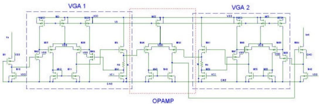
**Figure 2.22:** The circuit schematic of the tunable current mirror with preferred VGA topology.
