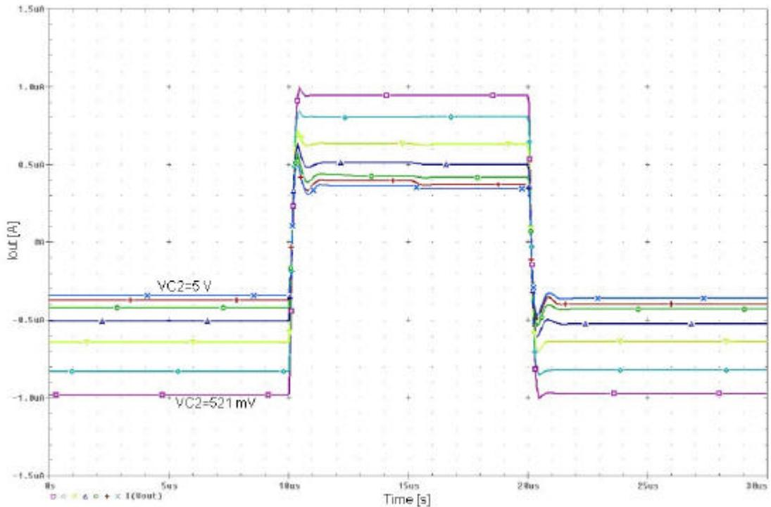
**Figure 2.36:** The pulse response of the tunable current mirror with VGAs for the compensated situation, obtained by changing  $V_{C2}$ .
