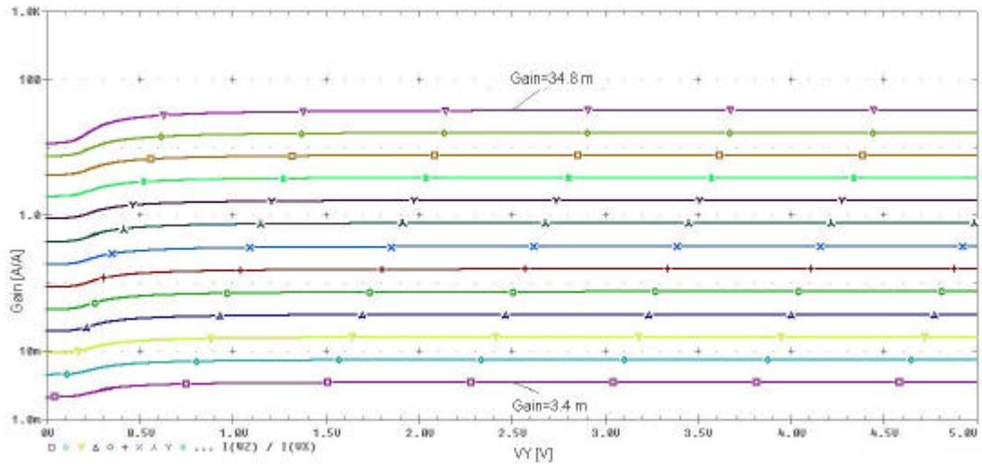
**Figure 2.66:** The change of the current gain of the ECCII according to  $V_C$ .
