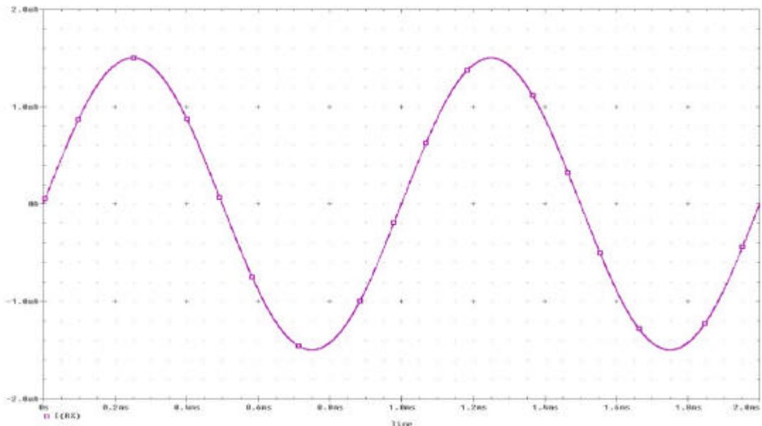
**Figure 2.68:**  $I_X$  current of the ECCII for sinusoidal voltage source applied to Y.
