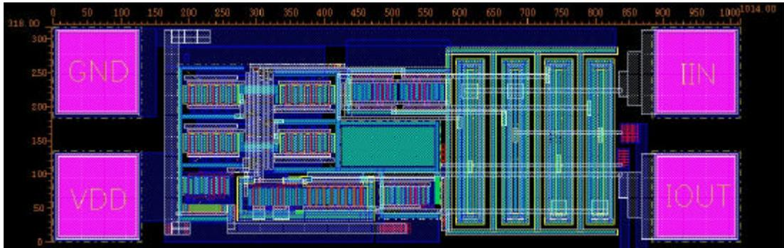
**Figure 2.52:** Layout of the tunable current mirror with current dividers circuit.
