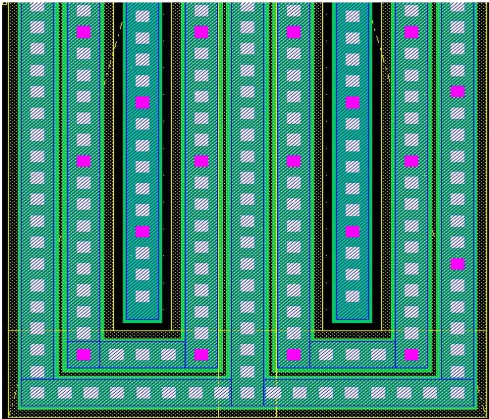
**Figure 2.53:** Layout of the parasitic PNP transistor.
