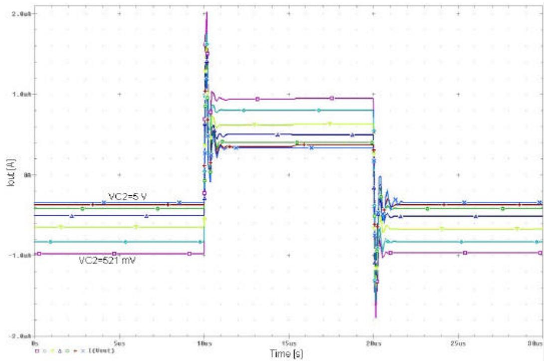
**Figure 2.35:** The pulse response of the tunable current mirror with VGAs for the uncompensated situation, obtained by changing  $V_{C2}$ .
