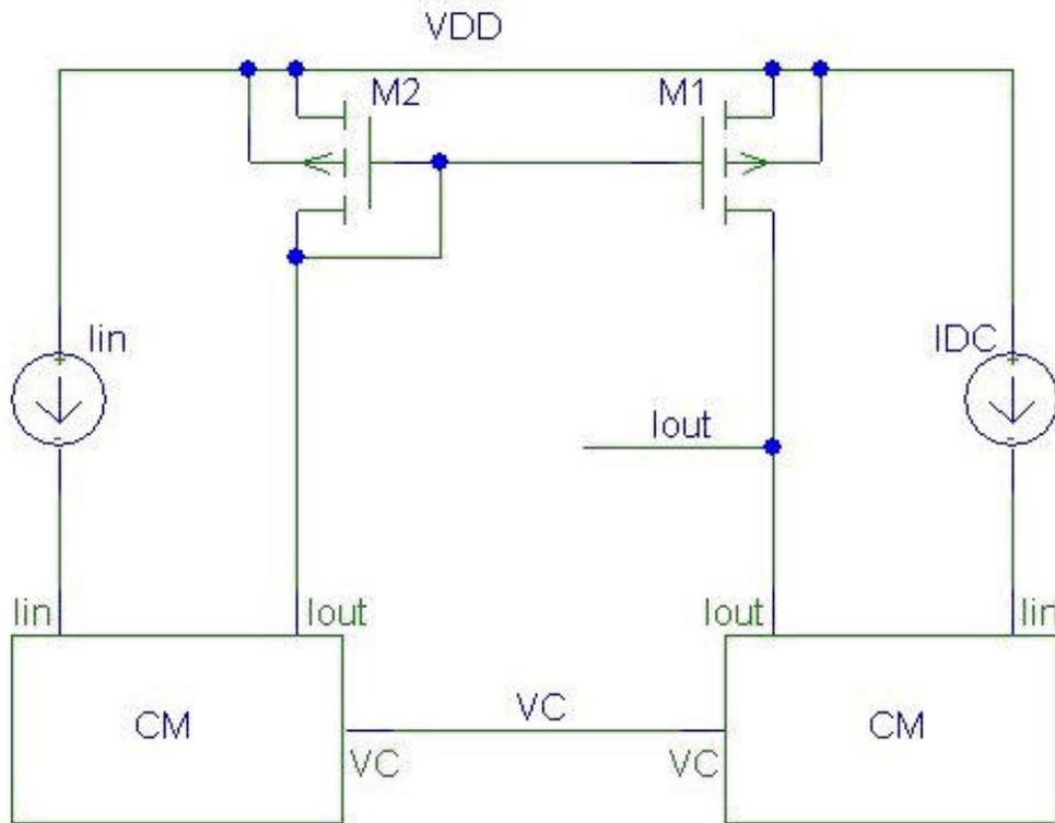
**Figure 2.17:** The configuration made to cancel the DC current component.
