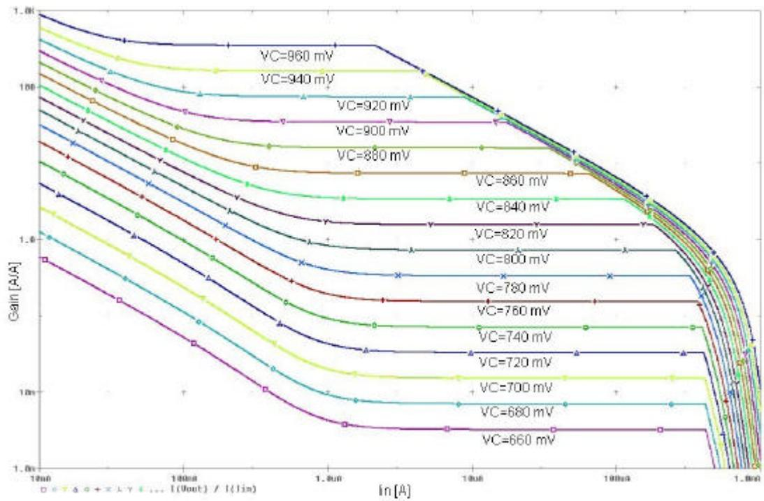
**Figure 2.55:** The change of the gain of the tunable current mirror with BJT differential pair for different  $V_C$  values.
