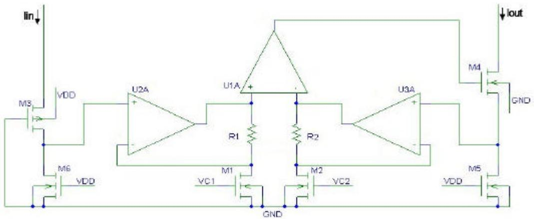
**Figure 2.21:** The tunable current mirror circuit with the preferred VGA topology.
