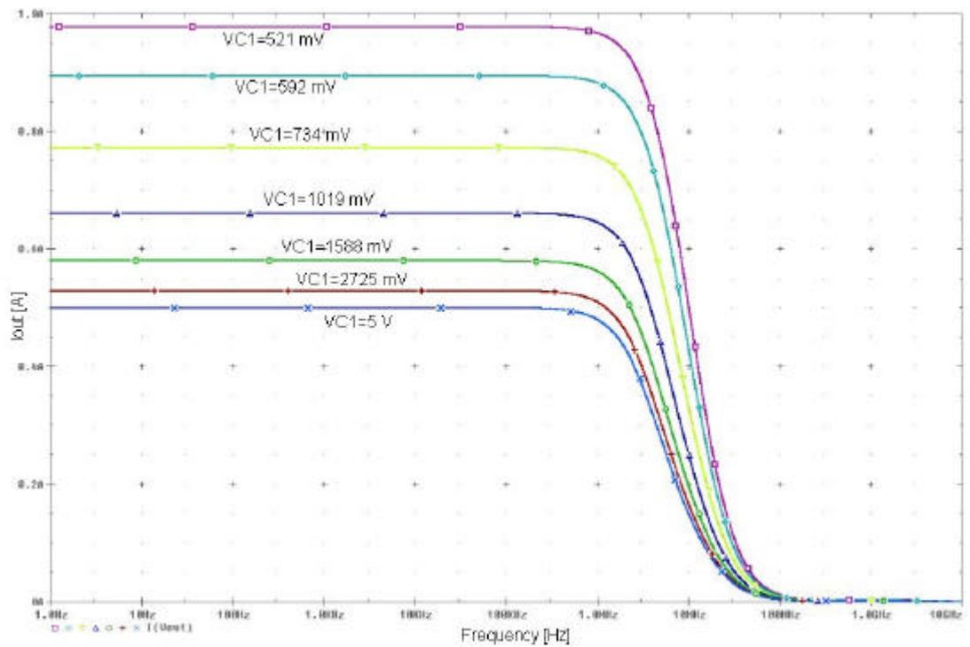
**Figure 2.13:** AC simulation result of the tunable current mirror with triode MOSFETs for different  $V_{C1}$  control voltage values.
