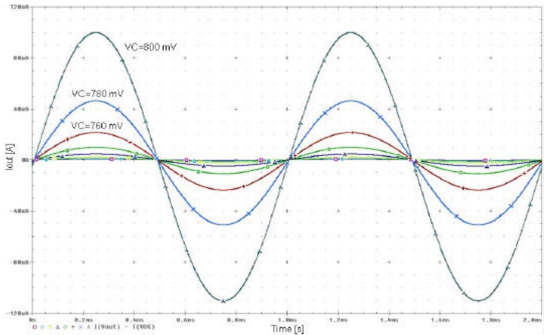
**Figure 2.59:** Transient simulation of the tunable current mirror with BJT differential pair with sinusoidal input for gains smaller than unity.
