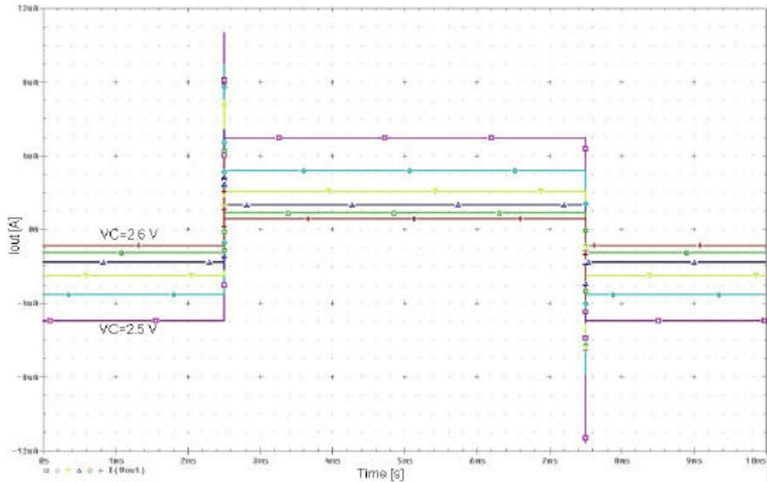
**Figure 2.50:** Pulse response of the tunable current mirror with current dividers in the uncompensated situation.
