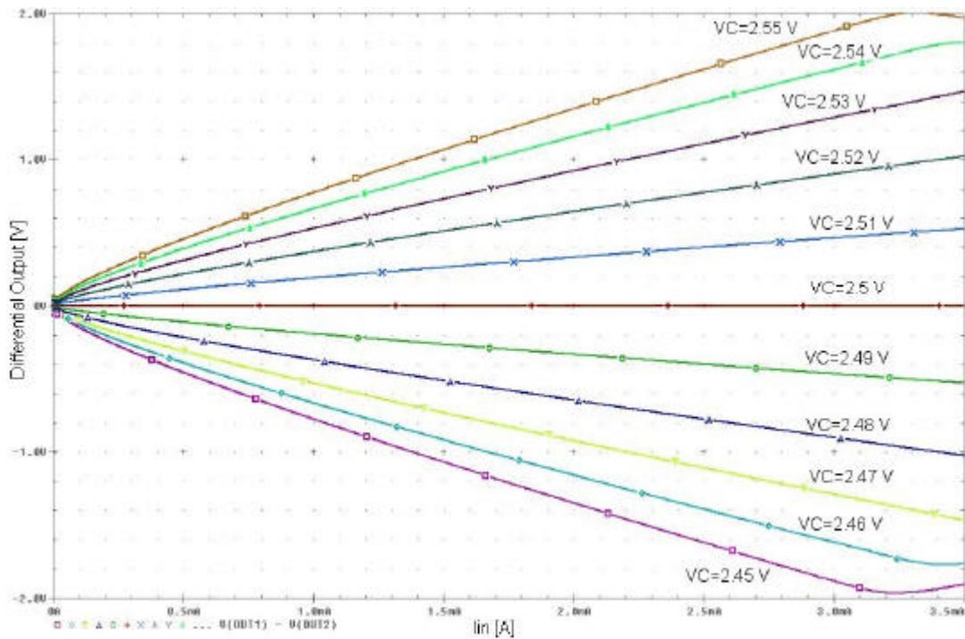
**Figure 2.39:** DC simulation result of the current divider.
