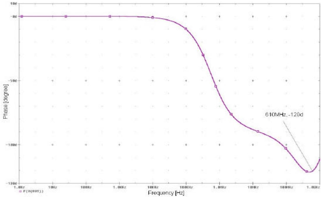
**Figure 2.7:** Phase response of the single stage opamp.
