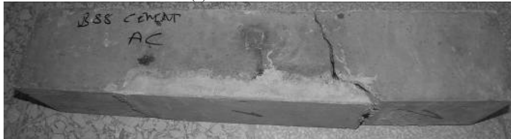
(b) Failure at the edge
