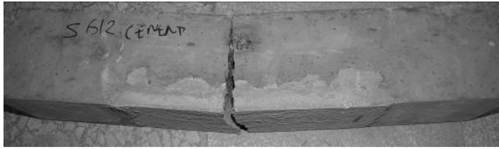
(a) Failure at the center
