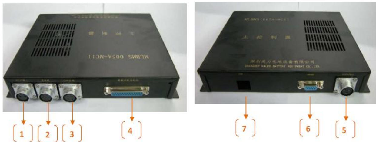
Figure 4.12: BMS Main Controller.
