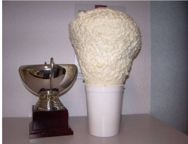
Figure 4.1 : Typical volume expansion of PU grouts
