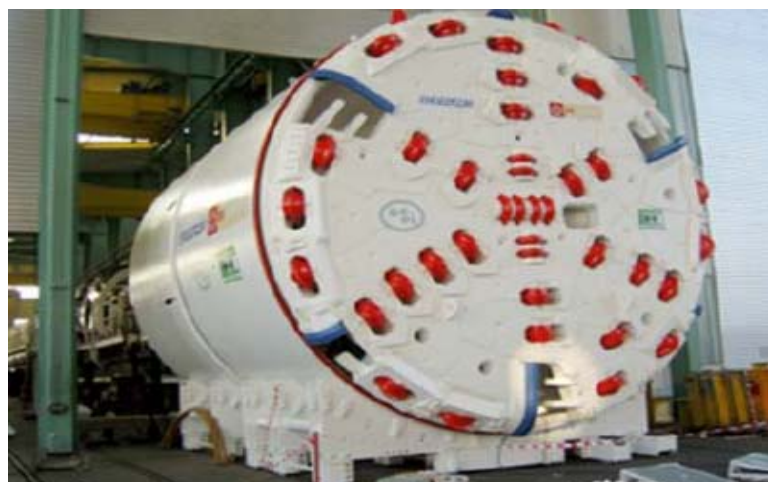
Figure 6.20 : Herrenknecht S-391 Hard Rock TBM (Melen Tunnel) [19].
