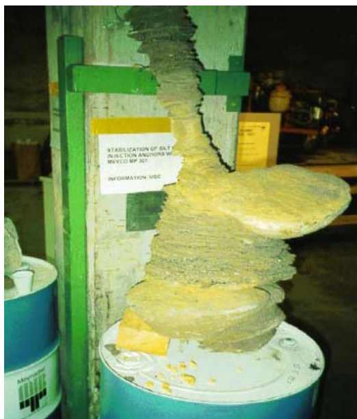
Figure 4.4 : Acrylic grout injected in sand.
