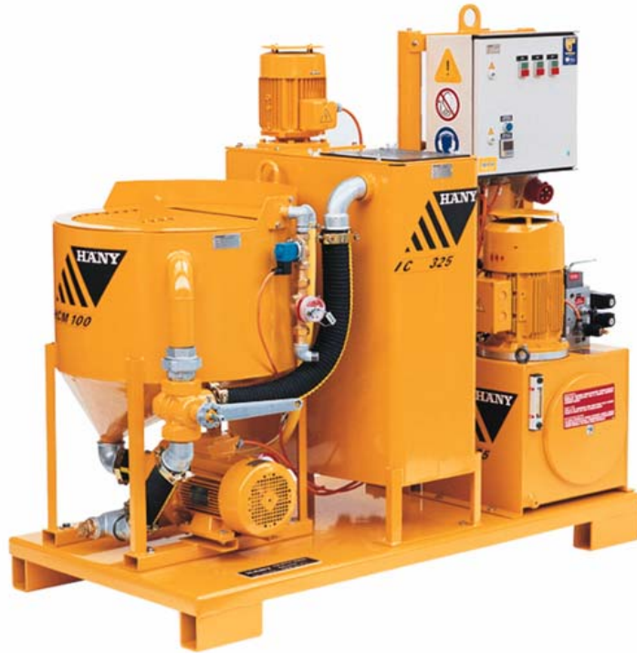
Figure 6.27 : Injection pump used for pre-injection grouting in Melen Tunnel.
