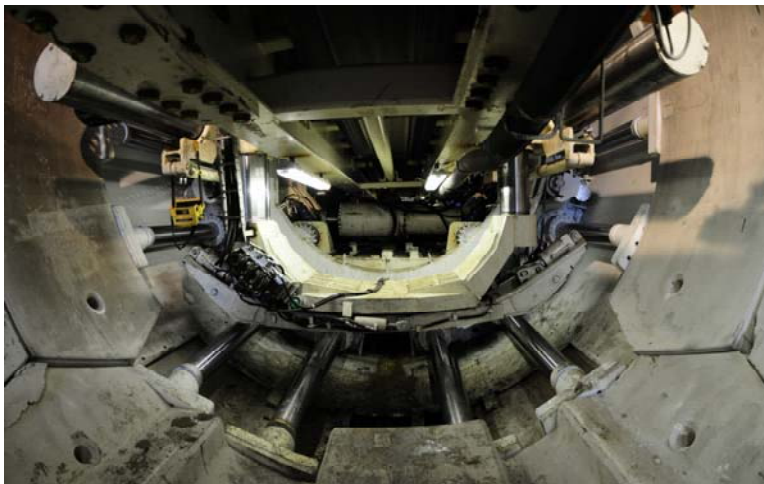
Figure 6.5 : Thrust cylinders of Mavi (Blue) Tunnel Double Shield TBM.
